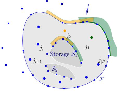
**Figure 6.** (a) An example of a setting in which the circular assumption holds. Squares indicate the witness points of  $\mathcal{W}$ . Jammers are indicated by disks. The portion of the fence and (boundary of) storage influenced by the orange jammer  $j_2$  (resp., green jammer  $j_1$ ) are highlighted in orange (resp., green). The arrow indicates a fence point influenced by both jammers.
