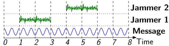
**Figure 2.** Jammers 1 and 2 actively transmit for the duration of two bits at different times during the transmission of a message. The transmissions of both jammers help to achieve the required bit-error probabilities.
