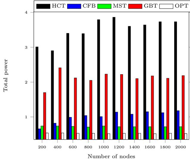
Figure 4: Total energy consumption in random networks. Comparing HCT ( $k = \sqrt{n}$ ), CFB, MST, GBT, and OPT (which is the optimal lower bound).
