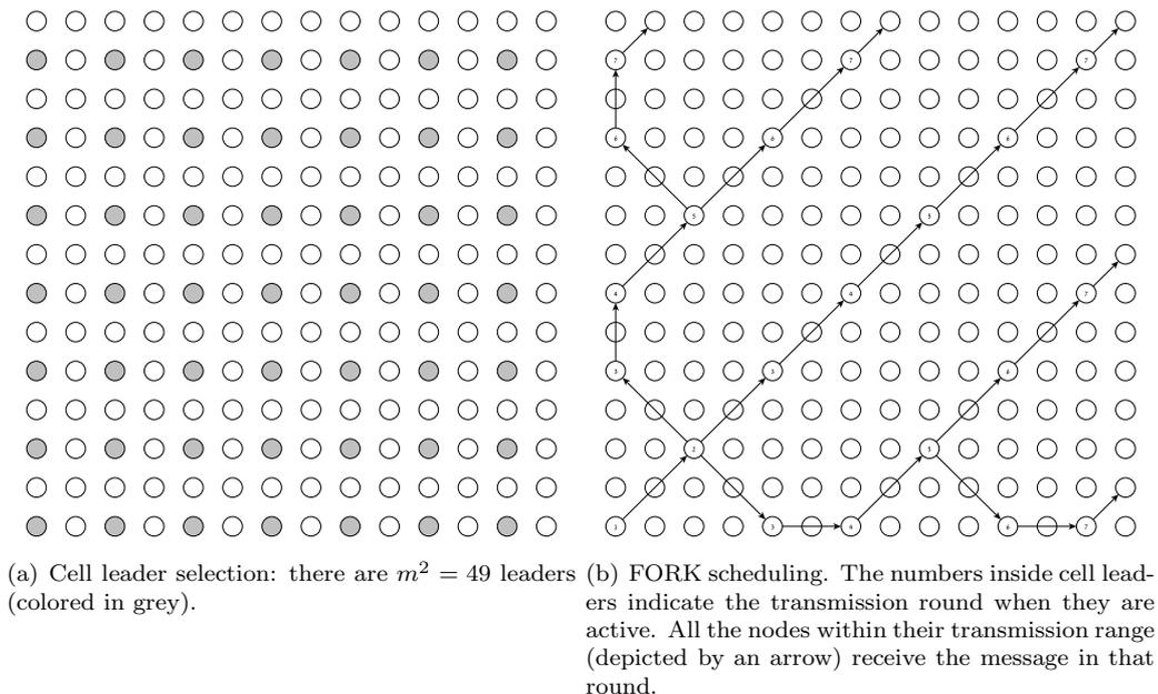
Figure 2: The FORK scheme with  $\sqrt{n} = 14$  and  $m = 7$ .
