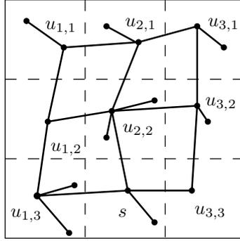
Figure 1: An example of GBT. There are 9 cells; the representative node in each cell,  $u_{i,j}$ , broadcasts to the nodes in the cell (the edges  $E_1$ ) and to the representatives of adjacent cells (the edges  $E_2$ ).
