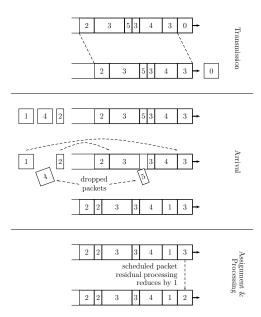
Fig. 1. An outline of the model. The top subfigure shows the transmission phase, the middle subfigure shows the arrival phase where packets might be discarded, and the bottom subfigure shows the assignment and processing phase. The length of a packet represents its size, and the number stamped on the packet represents the number of its (residual) required processing cycles.
