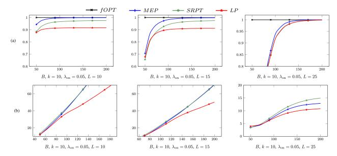
Fig. 5. Throughput performance (a) and latency (b) as a function of buffer size B for three different values of maximal packet length L.
