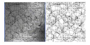
Fig. 2. VG of 450 RSs (10m antenna heights and 10 km transmission range). On the left: VG displayed over  $100 \times 100 km^2$  DEM (the lighter the higher). On the right: the same VG displayed with the DEM hidden.)
