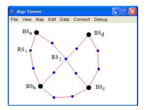
Fig. 1. Four BSs (big circles) and 11 RS (small circles) example: The optimal solution is 5 (using the middle RS), while any solution based on shortest path like method is 6 (using the outer RSs).
