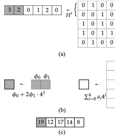
Fig. 6. Encoding of a systematic code with  $t = 1$  and  $\ell = 3$ .
