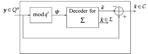
Fig. 2. Decoding asymmetric  $\ell$ -limited-magnitude error-correcting codes.
