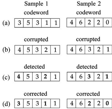
Fig. 1. Example of correcting asymmetric limited-magnitude errors.
