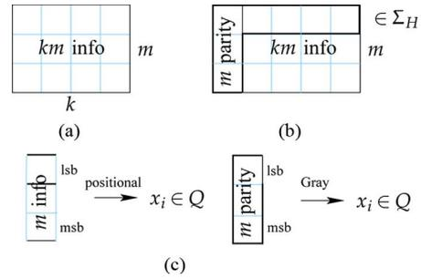
Fig. 5. Encoding procedure for a systematic code.
