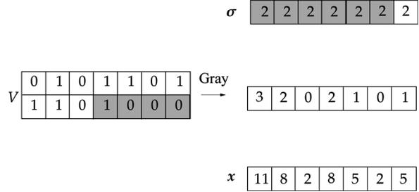
Fig. 8. Example of a code for asymmetric and symmetric limited-magnitude errors. From top to bottom: a codeword  $\sigma$  of the ternary repetition code; a binary Hamming codeword arranged into a  $2 \times 7$  array and its Gray mapping; the final codeword  $\mathbf{x}$  obtained by combining  $\sigma$  and  $V$ .
