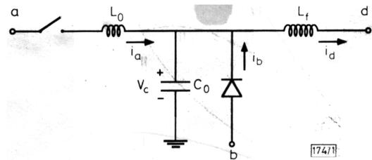
Fig. 1 Resonant switched-inductor model
