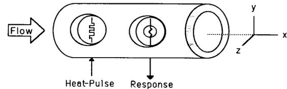
Fig. 1. Schematic representation of the thermal pulse flowmeter.
