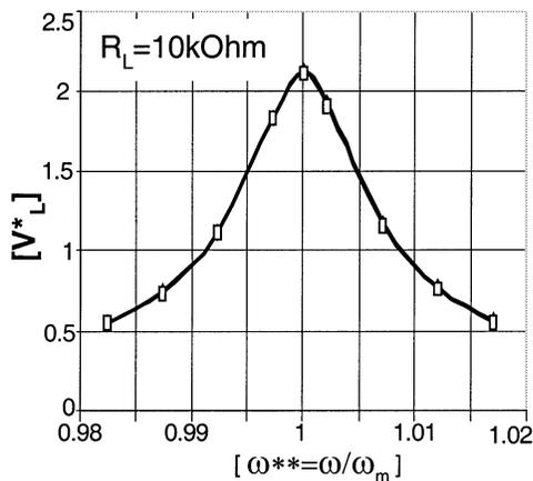
Fig. 10. Influence of operating frequency  $\omega$  on the normalized load voltage  $V_L^*$ . Solid line—ac model simulation,  $\square$ —cycle-by-cycle simulation. Load resistance  $R_L = 10 k\Omega$ .  $\omega_m$ —operating frequency corresponding to the maximum load voltage  $V_{Lmax}^*$ .
