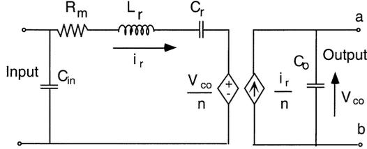
Fig. 2. Equivalent circuit of a piezoelectric transformer (PZT).
