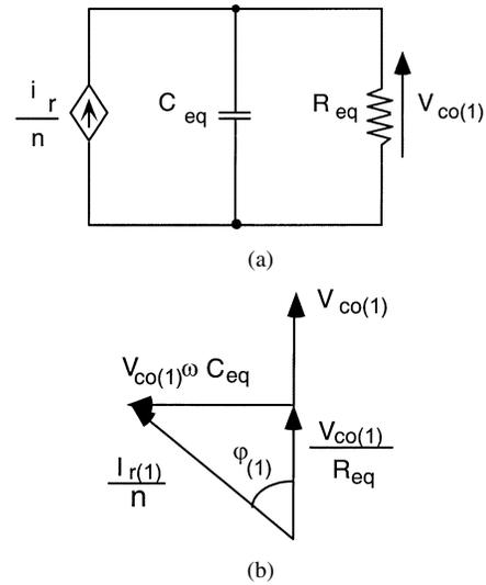
Fig. 5. Equivalent  $R_{eq} C_{eq}$  circuit replacing the reflected rectifier-load network fed by the current  $(I_r/n)$ : (a) topology and (b) vector diagram.
