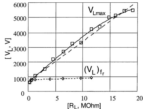
Fig. 12. Load voltage as a function of the load resistance  $R_L$ . Experimental data (points) and theoretical model (broken lines).  $(V_L)_{fr}$ —voltage corresponding to the resonant frequency  $f_r$ ;  $V_{Lmax}$ —maximum output voltage reached by frequency adjustment.
