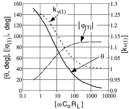
Fig. 4. Rectifier conduction angle  $\theta$ , the phase angle  $\varphi_{(1)}$  and the voltage waveform coefficient  $k_{v(1)}$  as functions of the load coefficient  $\omega C_o R_L$ .
