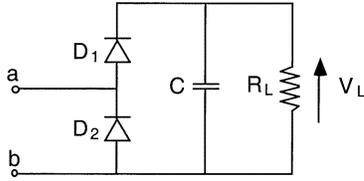
Fig. 1. Non-symmetrical topology of a voltage-doubler rectifier.
