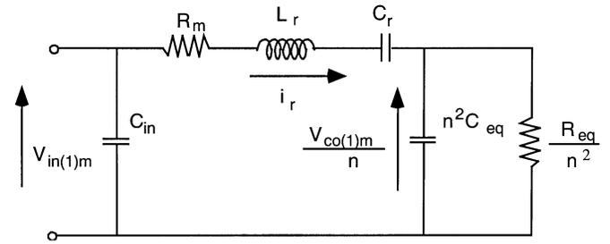
Fig. 7. AC equivalent circuit of the system: PZT, output rectifier and load.
