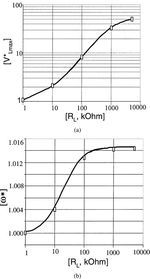
Fig. 9. Normalized maximum load voltage  $V_{Lmax}^*$  (a) and the corresponding normalized operating frequency  $\omega^*$  (b) as a function of the load resistance  $R_L$ . Solid lines—simulation (ac model) and analytical results;  $\square$ —results of cycle-by-cycle simulation.
