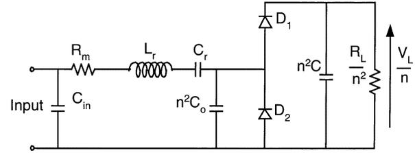
Fig. 8. AC/DC equivalent circuit of the system: PZT-voltage doubler rectifier.
