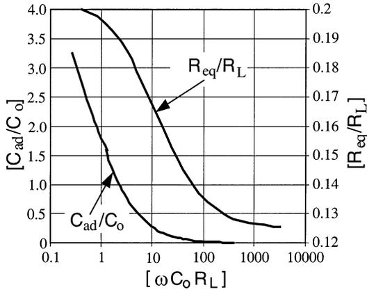
Fig. 6. Equivalent load resistance  $R_{eq}$  (pu) and apparent additional capacitance  $C_{ad}$  (pu) as functions of the load coefficient  $\omega C_o R_L$ .
