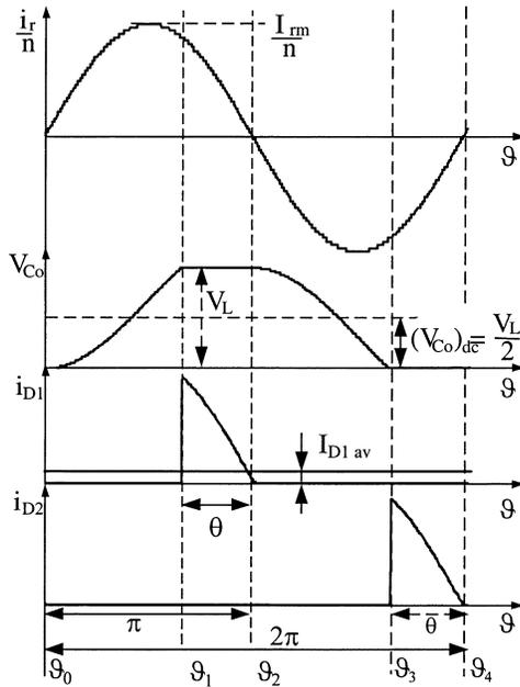
Fig. 3. Simulated current and voltage waveforms of the voltage doubler rectifier (Fig. 1) fed by a piezoelectric transformer (Fig. 2).
