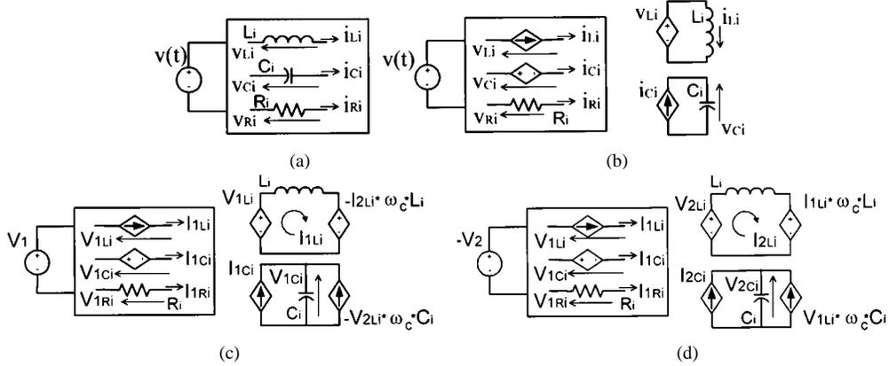
Fig. 1. Derivation of phasor equivalent circuits. (a) Original circuit. (b) Replacing reactive elements by dependent sources. (c) Real part of phasor equivalent circuit. (d) Imaginary part of phasor equivalent circuit.
