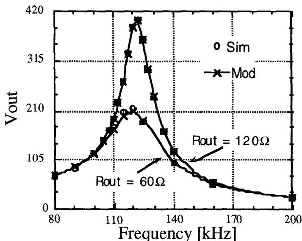
Fig. 5. Comparisons between the DC gain results of model simulation (Mod) and the cycle by cycle simulation (Sim) for  $R_{out} = 120\Omega$  and  $R_{out} = 60\Omega$ .
