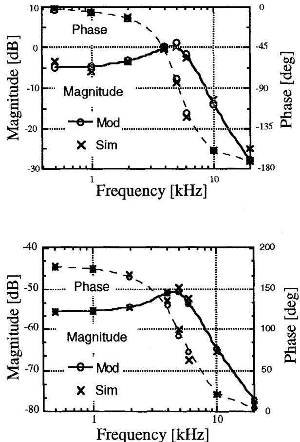
Fig. 8. Comparisons between small signal responses. Upper traces: switching frequency to output voltage response. Lower traces: Line to output voltage response (constant switching frequency:  $f_s = 160\text{kHz}$ ). Model simulation (Mod): circles. Cycle by cycle simulation (Sim): crosses.
