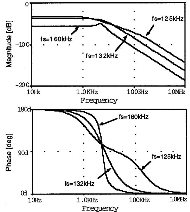
Fig. 7. Small signal, switching frequency to output voltage response for different center frequencies as obtained by the proposed model.
