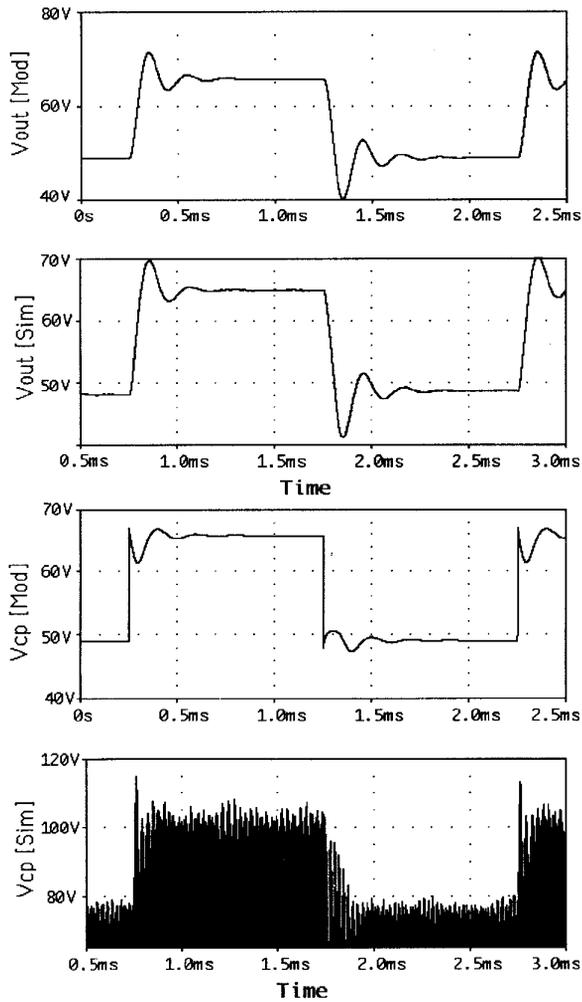
Fig. 6. Comparisons between  $V_{out}$  (Upper two traces) and  $V_{cp}$  (Lower two traces) response to a step in frequency. Upper traces: model simulation (Mod); Lower traces: cycle by cycle simulation (Sim).
