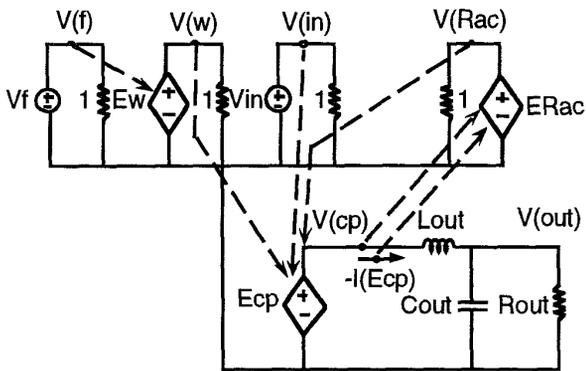
Fig. 3. Average model of the series-parallel resonant converter by applying PSPICE (Micro Sim Inc) behavioral dependent sources.
