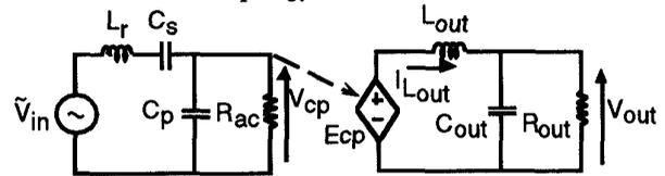
Fig. 2. First-harmonic approximation of the series-parallel resonant converter.
