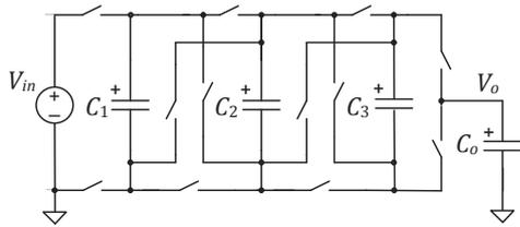
Fig 11: Switch network used in the binary SCC.
