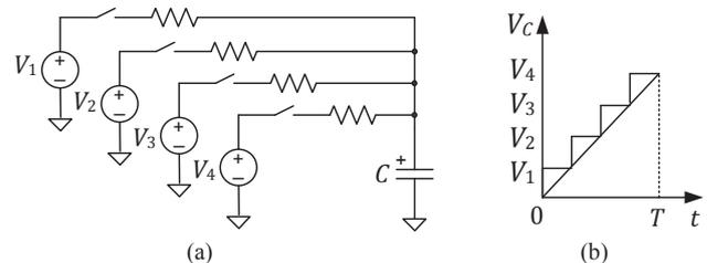
Fig. 2: Stepwise charging of a capacitor by multiple voltage sources (a) and the resulting stepped voltage (b).
