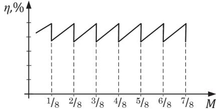
Fig. 4: Theoretical efficiency of the binary SCC.
