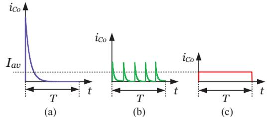
Fig. 7: Possible forms of momentary current through  $C_o$ .
