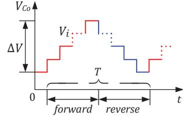
Fig. 6: Voltage across  $C_o$  in the proposed approach.
