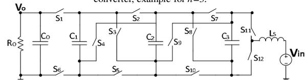
Fig. 3: Resonant Binary/Fibonacci switched capacitor step-up converter, example for  $n=3$ .
