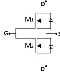
Fig. 5: Bi-directional switch using N-channel power MOSFETs.
