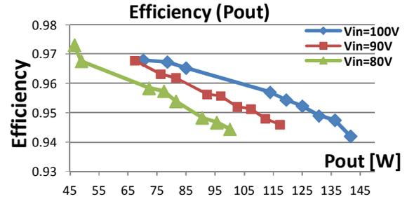
Fig. 14: Efficiency of step-down, Resonant Binary SCC,  $M=5/8$ .
