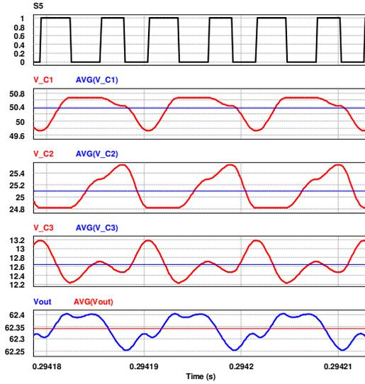
Fig. 10: Capacitors and output voltages waveforms,  $M=5/8$ .
