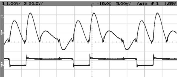
Fig. 12:  $I_{out}$  and  $V_{DS}(S6)$  at  $V_{in}=80V$ ,  $P_{out}=100W$ ,  $M=5/8$ .
