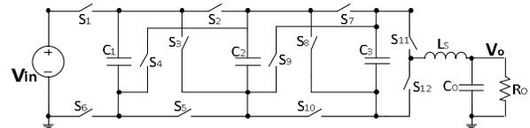
Fig. 2: Resonant Binary/Fibonacci switched capacitor step-down converter, example for  $n=3$ .
