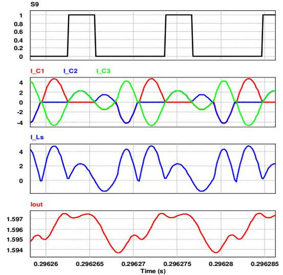
Fig. 9: Capacitors and output stage current waveforms,  $M=5/8$ .
