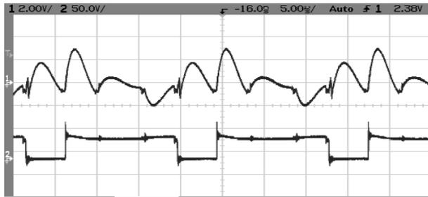
Fig. 11:  $I_{out}$  and  $V_{DS}(S6)$  at  $V_{in}=100V$ ,  $P_{out}=136W$ ,  $M=5/8$ .
