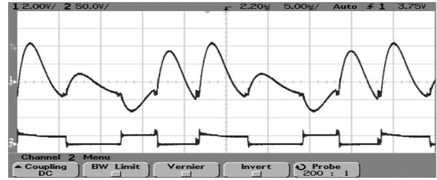
Fig. 13:  $I_{out}$  and  $V_{DS}(S6)$  at  $V_{in}=60V$ ,  $P_{out}=69.89W$ ,  $M=3/8$ .
