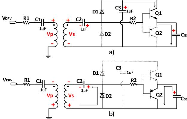
Fig. 7: Operation modes: a) ON state -  $C_{GS}$  charging.
