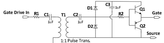
Fig. 6: The Isolated Gate Driver.
