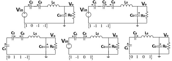
Fig 4: Resonant SCC topologies configured from the EXB codes of  $M=5/8$ .
