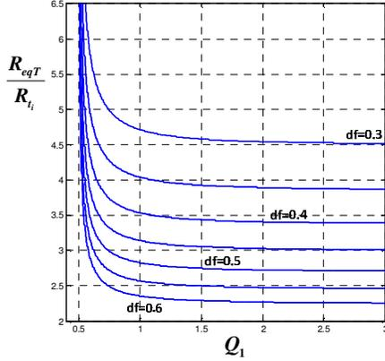
Fig. 8: Dependence of the normalized equivalent resistance on the Quality factor ( $Q_1$ ) and the frequency ratio, ( $df_i$ ).
