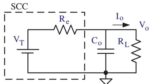
Fig. 1. Generic SCC model for loss evaluation.
