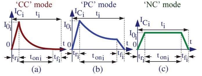
Fig. 5. Possible variants of capacitor current waveforms when the charge or discharge process is: (a) Complete ( $T_i \gg R_i C_i$ ); (b) Partial ( $T_i \cong R_i C_i$ ); (c) 'No Charge' ( $T_i \ll R_i C_i$ ).
