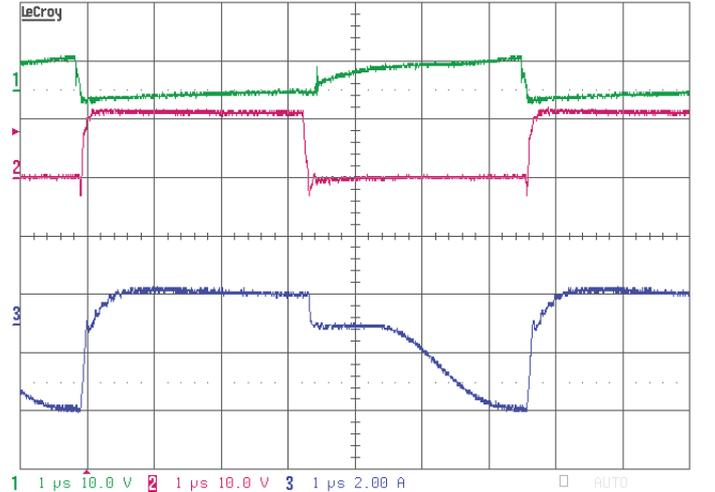
Fig. 7. Experimental waveforms in the 'NC' mode,  $T_i \ll R_i C_i$ ,  $f_s = 150 \text{ kHz}$ : Upper trace –  $S_2$  gate signal, discharging switch; Middle trace –  $S_1$  gate signal, charging switch; Lower trace - Flying capacitor current.
