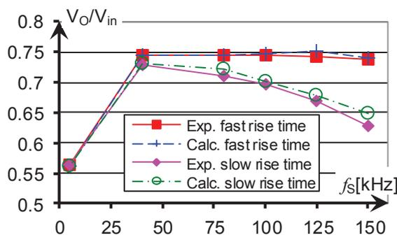
Fig. 9. Output voltage at different operational modes. Experimental results (lines): Square marks - fast rise times, diamond marks - slow rise times. Model calculation results (dashed lines): Plus marks - fast rise times, circle marks - slow rise times.
