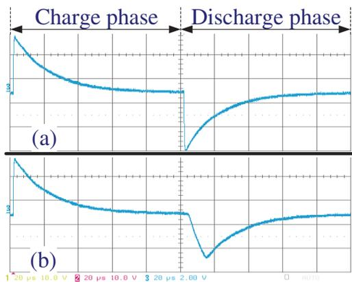
Fig. 8. Flying capacitor current waveforms in 'CC' mode with a different rise time in the discharge phase: (a) Fast rise time,  $V_O = 5.63V$ ; (b) Slow rise time,  $V_O = 5.63V$ .
