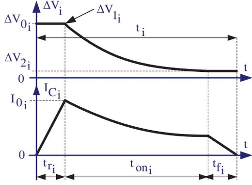
Fig. 6. Detailed waveforms of the 'PC' mode ( $T_i \cong R_i C_i$ ): Upper trace: voltage  $\Delta V_i$  across resistance  $R_i$  and  $S$ ; Lower trace: current through the capacitor, according to the notations in Fig. 4.
