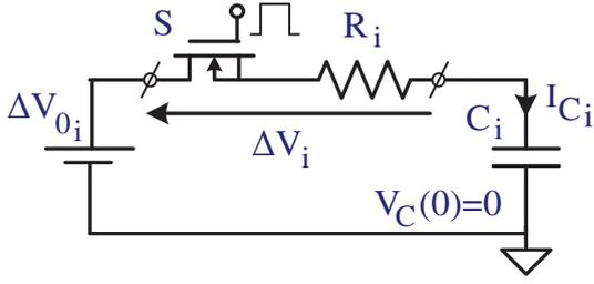
Fig. 4. Equivalent circuit of a charge ( $i = 1$ ) or discharge ( $i = 2$ ) process.
