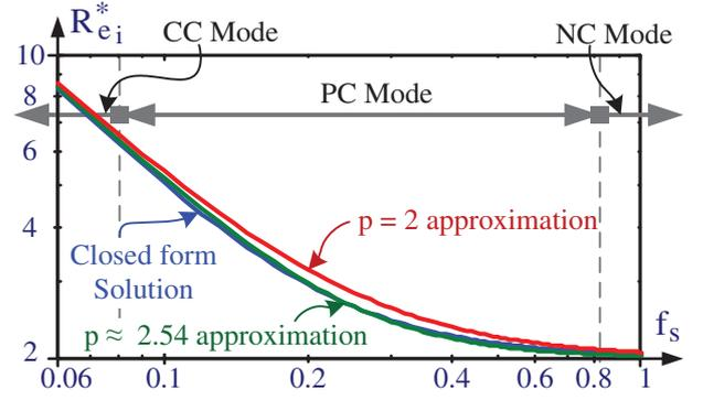
Fig. 2. Comparison of two empirical approximations of equivalent resistance to the closed form solution.
