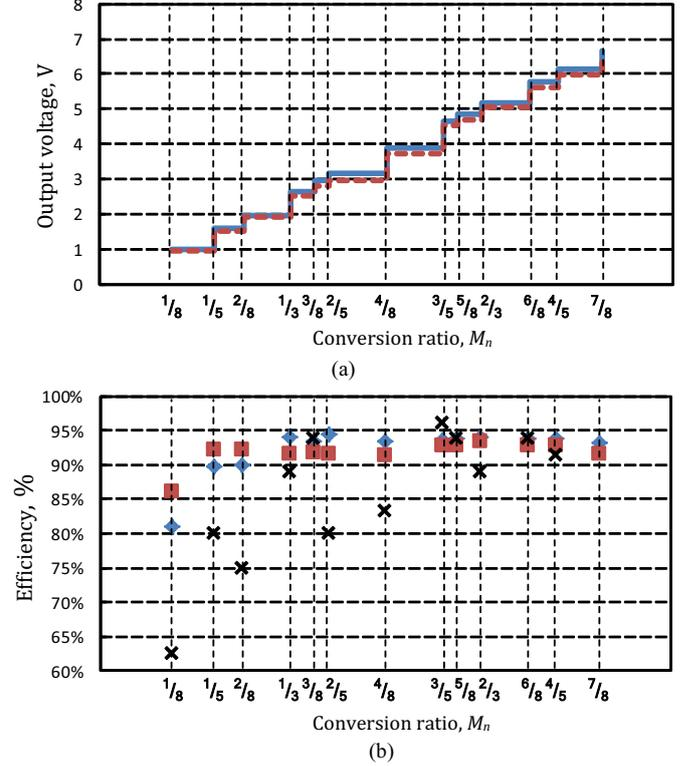
Fig. 7: The output voltage (a) and efficiency (b) of the experimental SCC. Diamonds:  $R_o=300\Omega$ . Squares:  $R_o=100\Omega$ . The curve of the higher output voltage in (a) is for  $R_o=300\Omega$ , while the one of the lower output voltage is for  $R_o=100\Omega$ . The points marked by "X" in (b) are estimates of minimum efficiency of a regulated version of proposed SCC in between target voltages.
