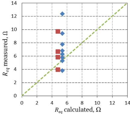
Fig. 8: Measured values of  $R_{eq}$  compared to the calculated ones. Diamonds:  $R_o=300\Omega$ . Squares:  $R_o=100\Omega$ .
