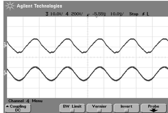
Fig. 11. Experimental waveforms: input phase current  $i_R$  (upper trace) and input phase voltage  $v_R$  (lower trace). Vertical scale (upper trace): 10A/div., Vertical scale (lower trace): 200V/div., horizontal scale: 10msec/div.. (See Fig. 8).
