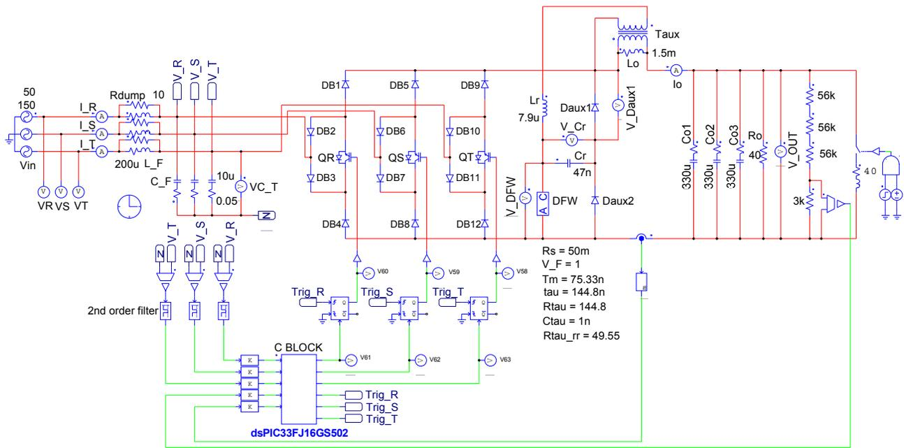
Fig. 8. Simulation and equivalent experimental circuit diagram of lossless turn-on snubber applied to a three-phase buck-type rectifier. The snubber inductor  $L_r$  is coupled to the main inductor  $L_o$ .
