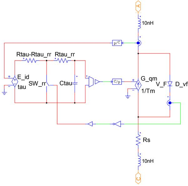
Fig. 2. Proposed diode model with reverse recovery (PSIM implementation). The 10nH inductor represents a parasitic lead inductance.
