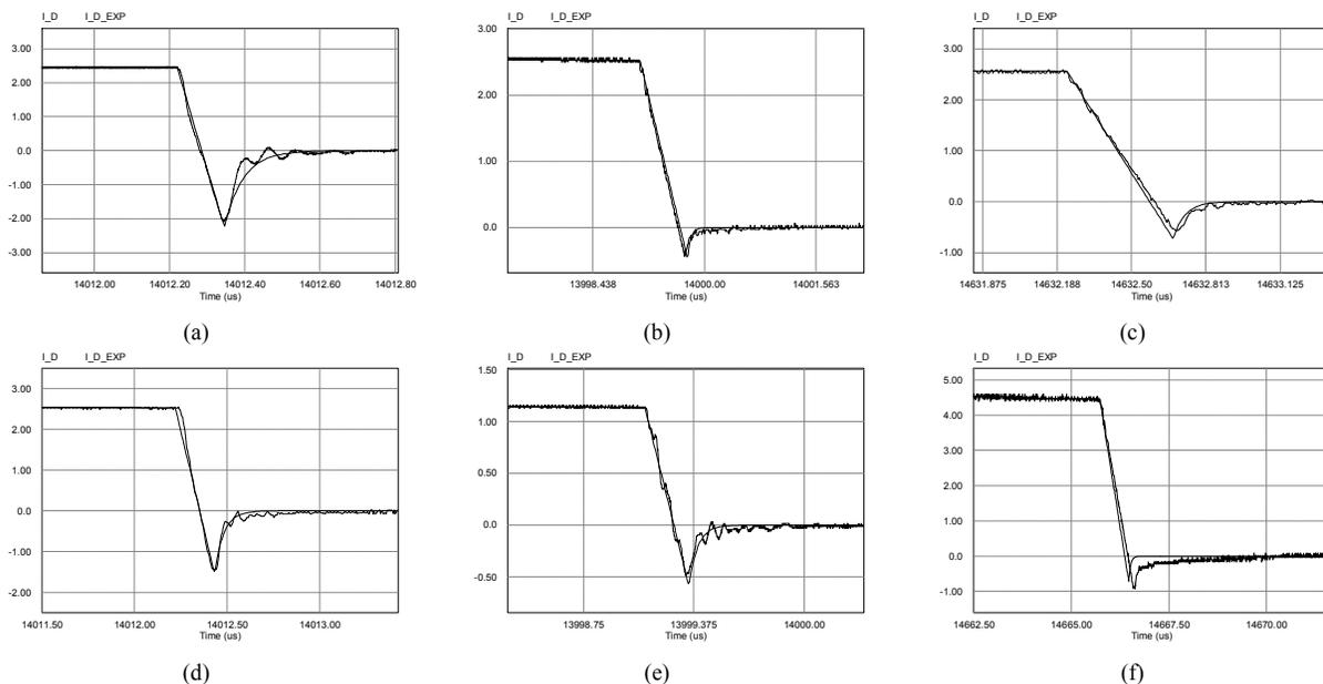
Fig. 5. Reverse recovery model validation (PSIM simulation). (a) Comparison to the measurement curve of Fig. 3, (b)  $L_r = 10\mu H$ ,  $I_F = 2.5A$ , (c)  $L_r = 6\mu H$ ,  $I_F = 2.5A$ , (d)  $L_r = 1.3\mu H$ ,  $I_F = 2.5A$ , (e)  $L_r = 6\mu H$ ,  $I_F = 1.3A$ , (f)  $L_r = 6\mu H$ ,  $I_F = 4.3A$ .
