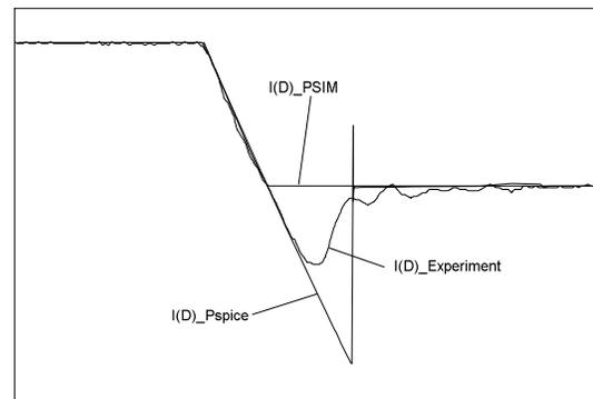
Fig. 1. Experimental and simulated turn-off current waveforms of a power diode (PSIM disregards reverse recovery process).
