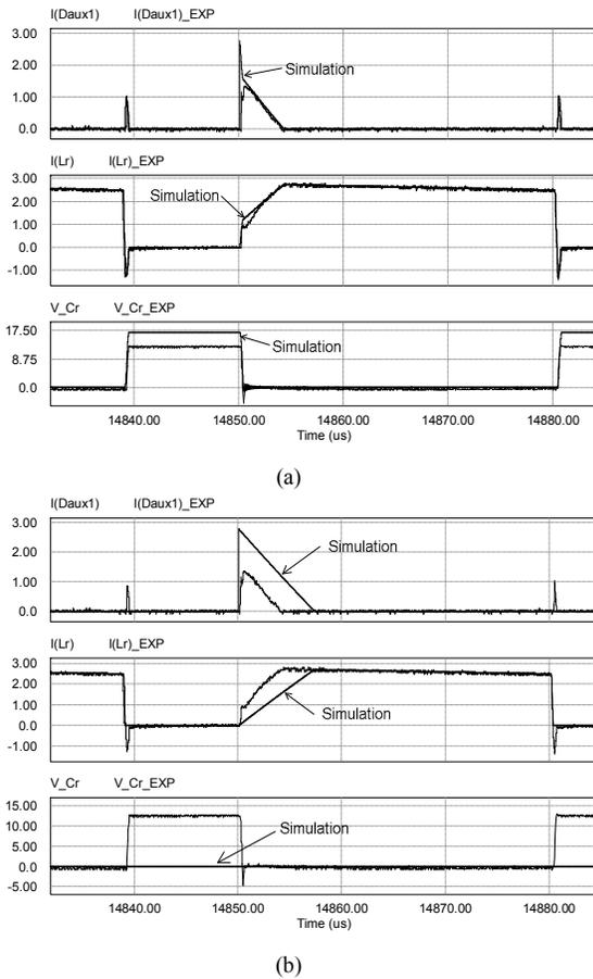
Fig. 7. Comparison between simulation (PSIM) and the experimental waveforms of the turn-on lossless snubber: (a) results when the proposed diode model is included, (b) the results when the original PSIM diode is used.
