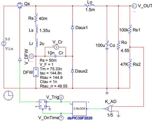
Fig. 6. Circuit diagram of simulation and experimental setup of dc-dc buck converter.  $L_r$  and  $L_s$  are the snubber inductor and stray inductance, respectively.
