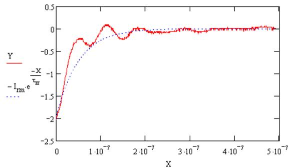
Fig. 4. Extracted reverse recovery time constant  $\tau_{rr}$ . Y is the measurement data during  $t > t_a$  and the dashed curve corresponds to the fitting of equation (4) with the following outcomes:  $I_{rm} = 2A$  and  $\tau_{rr} = 49.55nsec$ .
