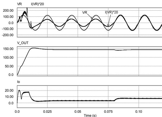
Fig. 9. AC side (top trace) and DC side (middle and bottom traces) simulated waveforms (PSIM) of the three-phase rectifier.
