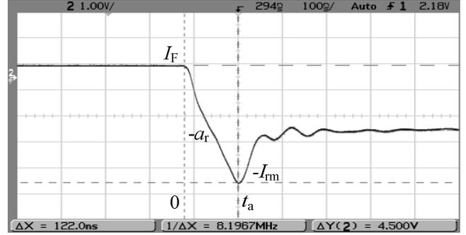
Fig. 3. Experimental turn-off current waveform of power diode (MUR8100E, ON-Semi) with stray inductance ( $L_s = 1.35\mu\text{H}$ ,  $I_f = 2.5\text{A}$ ,  $I_{rm} = 2\text{A}$ ,  $a_r = \Delta Y/\Delta X$ ,  $t_a = \Delta X$ ). Vertical scale: 1A/div., horizontal scale: 100nsec/div..
