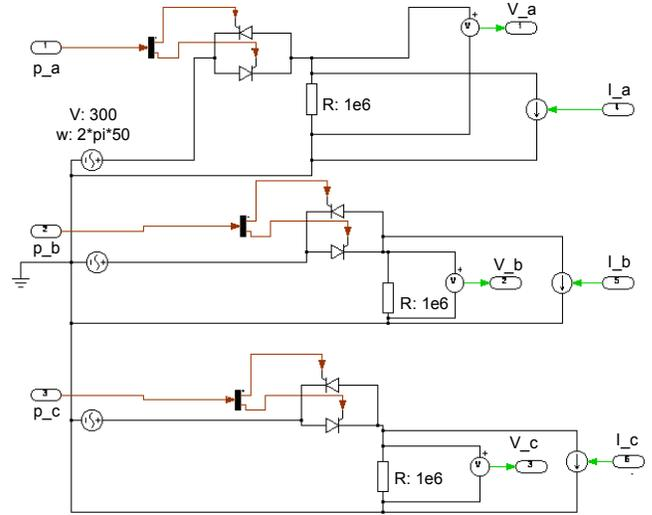
Fig. 12. The contents of the Plecs block.
