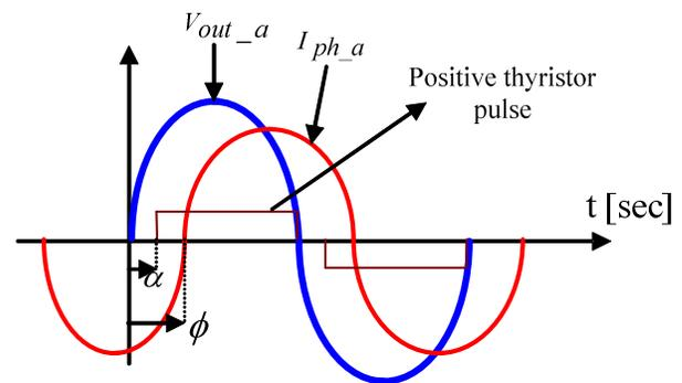
Fig. 2. The waves of phase voltage  $V_{out\_a}$  and current  $I_{ph\_a}$  in continuous mode ( $\phi = 75^\circ, \alpha = 40^\circ, \gamma = -35^\circ$ ).
