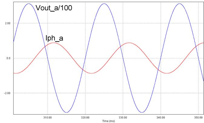
Fig. 9. Psim simulated phase 'a' voltage-  $V_{out\_a}/100$  [v] and the phase 'a' current  $I_{ph\_a}$  [A], for  $\alpha=110^\circ$ ,  $n=1533$  rpm, "star" connection. (X- 10 msec/div, Y1- 100V/div, Y2- 1A/div)
