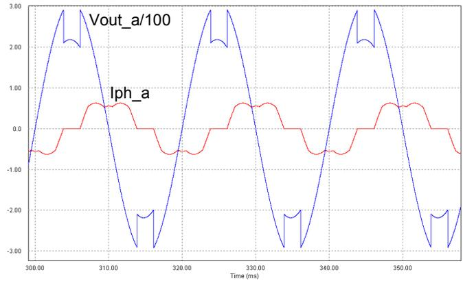
Fig. 8. Psim simulated phase voltage of the machine-  $V_{out\_a}/100$  [V] and the phase current  $I_{ph\_a}$  [A], for  $\alpha=110^\circ$ ,  $n=1500$  rpm, "star" connection. (X- 10 msec/div, Y1- 100V/div, Y2- 1A/div)
