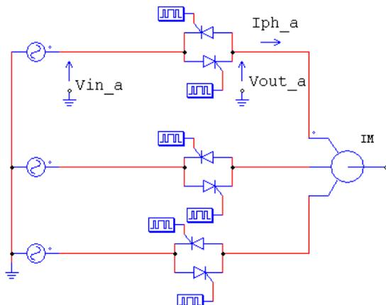
Fig. 1. Induction machine (star connection) controlled by thyristors.
