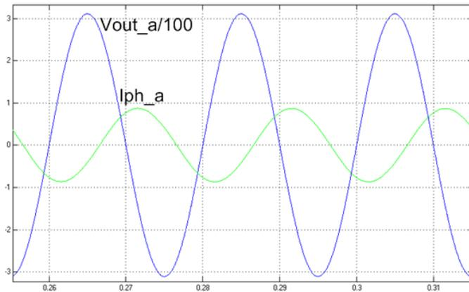
Fig. 14. Plecs simulated phase voltage of the machine-  $V_{out\_a}/100$  [V] and the phase current  $I_{ph\_a}$  [A], for  $\alpha = 110^\circ$ ,  $n=1533$  rpm, “star” connection. (X- 10 msec/div, Y1- 100V/div, Y2- 1A/div)
