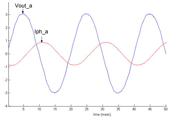
Fig. 16. Measured phase voltage of the machine-  $V_{out\_a}/100$  [V] and the phase current  $I_{ph\_a}$  [A], for  $\alpha = 110^\circ$ ,  $n=1533$  rpm, “star” connection.
