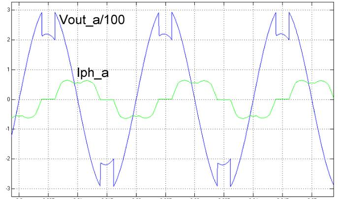
Fig. 5. Simulink simulated phase voltage of the machine-  $V_{out\_a}/100$  [V] and the phase current  $I_{ph\_a}$  [A], for  $\alpha = 110^\circ$ ,  $n = 1500$  rpm, "star" connection. (X- 5 msec/div, Y1- 100V/div, Y2- 1A/div)
