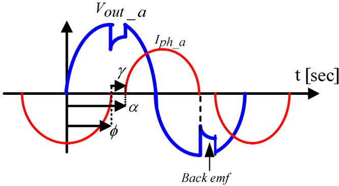
Fig. 3. The waves of phase voltage  $V_{out\_a}$  and current  $I_{ph}$  in discontinuous mode ( $\phi = 80^\circ$ ,  $\alpha = 100^\circ$ ,  $\gamma = 20^\circ$ ).
