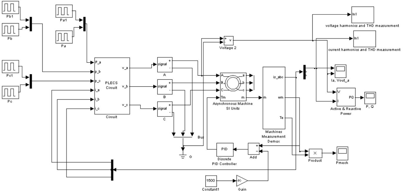
Fig. 11. The Plecs and Simulink co-simulation file.
