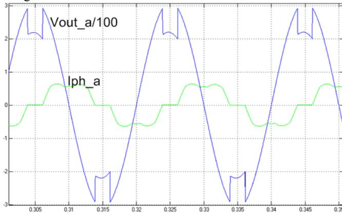
Fig. 13. Plecs simulated phase voltage of the machine-  $V_{out\_a}/100$  [V] and the phase current  $I_{ph\_a}$  [A], for  $\alpha = 110^\circ$ ,  $n=1500$  rpm, “star” connection. (X- 5 msec/div, Y1- 100V/div, Y2- 1A/div)
