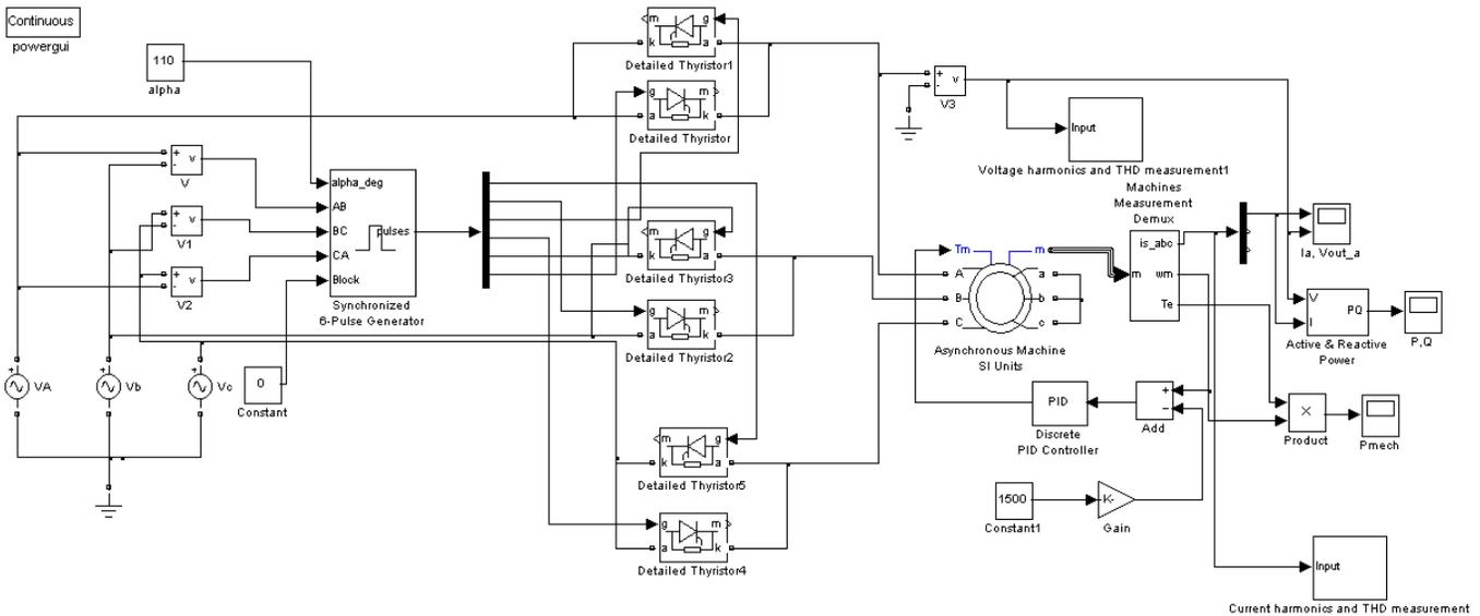
Fig. 4. The Simulink simulation circuit for "star" connected stator.
