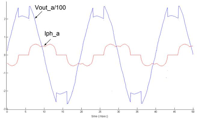
Fig. 15. Measured phase voltage of the machine-  $V_{out\_a}/100$  [V] and the phase current  $I_{ph\_a}$  [A], for  $\alpha = 110^\circ$ ,  $n=1500$  rpm, “star” connection.
