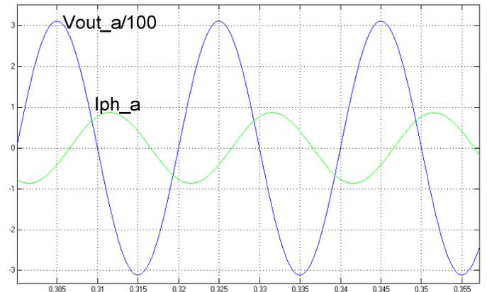
Fig. 6. Simulink simulated phase 'a' voltage-  $V_{out\_a}/100$  [v] and the phase 'a' current  $I_{ph\_a}$  [A], for  $\alpha = 110^\circ$ ,  $n = 1533$  rpm, "star" connection. (X- 5 msec/div, Y1- 100V/div, Y2- 1A/div)
