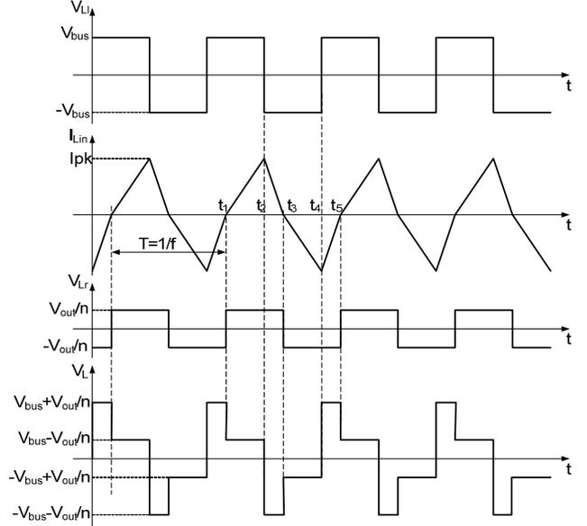
Figure 2. Basic waveforms of the proposed inverter. From top to bottom:  $V_{L1}$ , Inductor current,  $V_{Lr}$ , voltage across inductor.
