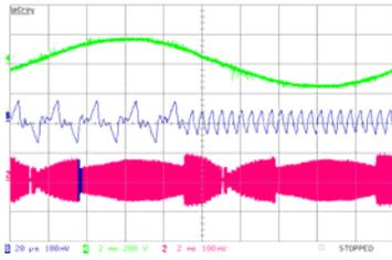
Figure 6. Inductor current over a line period. Lower trace: inductors current 5A/div; Middle trace: zoom-in of the marked zone of the lower trace 5A/div. Upper trace: line voltage 200V/div; Horizontal scale: upper and lower traces - 2ms/div; middle trace - 20µs/div.
