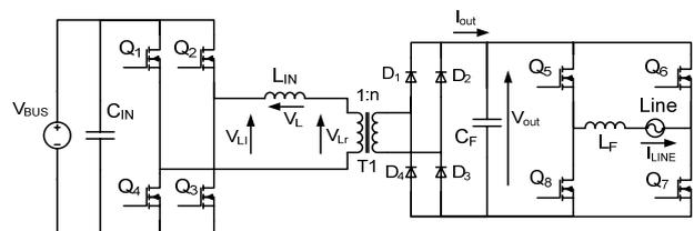
Figure 1. The proposed grid connected inverter.
