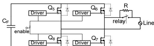
Figure 7. Output bridge and grid connecting circuitry.
