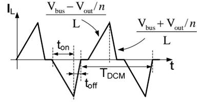
Figure 4. Inductor's current at PWM mode of operation.
