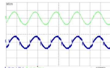
Figure 5. Output behavior of the inverter with no sensing of the output voltage.  $V_{in}=115V$ ;  $V_{line}=110V_{rms}$ ;  $P_{out}=150W$ . Upper trace: line current ( $I_{LINE}$ ) 2A/div; Lower trace: line voltage 200V/div; Horizontal scale: 20ms/div.
