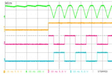
Figure 8. Grid connection sequence.  $V_{line}=110V$ ; From top to bottom: capacitor's voltage 100V/div; "enable" signal of the output inverter 5V/div; gate signal to one diagonal of the output bridge 5V/div; gate signal to another diagonal of the output bridge 5V/div; Horizontal scale: 10ms/div.
