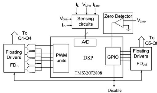
**Figure 5:** DSP based control circuit of the proposed OCS inverter
