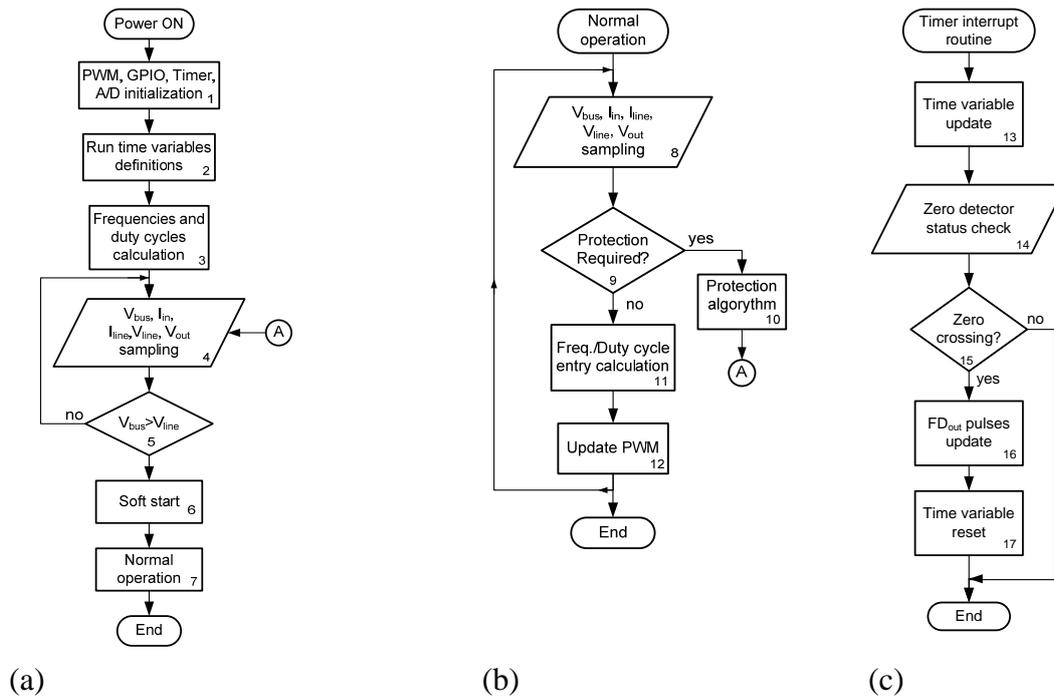
**Figure 6:** Block diagram of control algorithm.
