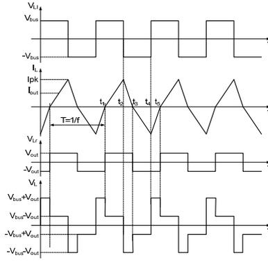
**Figure 2:** Basic waveforms of the proposed inverter, for  $n=1$ .
