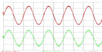
**Figure 7:** Output behavior of the inverter with no sensing of the output voltage.
