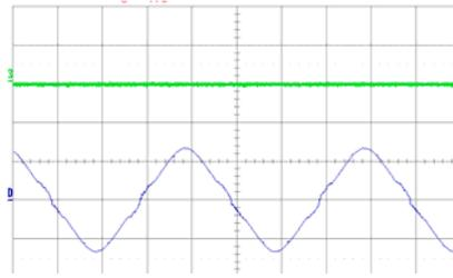
**Figure 8:** Output current of the inverter with shorted output.  $V_{in}=265V$ ;
