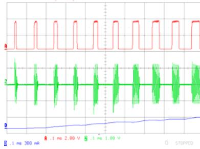
**Figure 4:** Dithering mode around zero cross.
