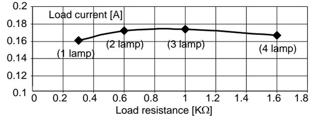
Figure 13. Experimental results, Load current as a function of the load resistance. Constant-current driver operation.
