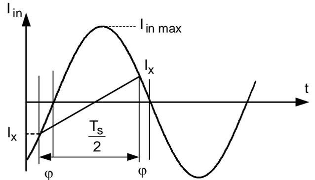
Figure. 6. The desired commutation intersection point, referred to the approximated input current.
