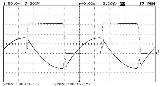
Figure 14. Experimental results, ZVS operation when loaded by 300Ω : top: drain voltage of  $Q_2$  (50V/div); bottom  $I_{out}$  (0.2A/div); Horizontal scale: 2μS/div
