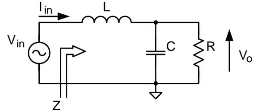
Figure 3. Equivalent circuit, simplified by first harmonic theorem
