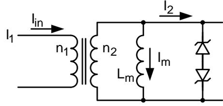
Figure 7. Current transformer, simplified circuit.
