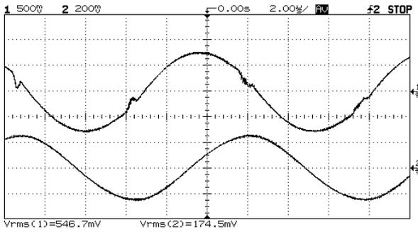
Figure 11. Experimental results, constant current when loaded by 1000Ω : top:  $I_{out}$  (0.2A/div); bottom  $I_{lamp}$  (0.2A/div); Horizontal scale: 2μS/div
