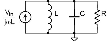
Figure 4. Equivalent parallel network by Norton's theorem
