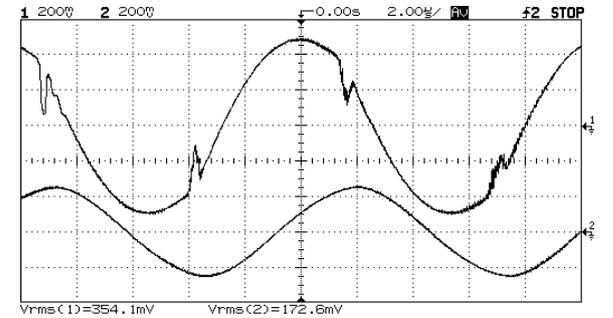
Figure 10. Experimental results, constant current when loaded by 600 $\Omega$  : top:  $I_{out}$  (0.2A/div); bottom  $I_{lamp}$  (0.2A/div); Horizontal scale: 2 $\mu$ S/div
