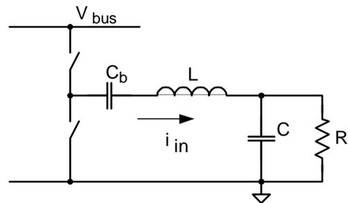
Figure 1. A half-bridge inverter feeding a resonant network
