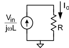
Figure 5. Equivalent parallel network by Norton's theorem at  $\omega = \omega_0$
