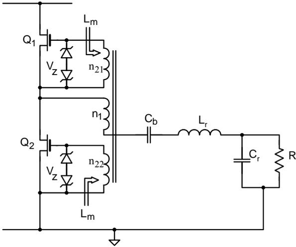
Figure 2. Self-Oscillating resonant inverter
