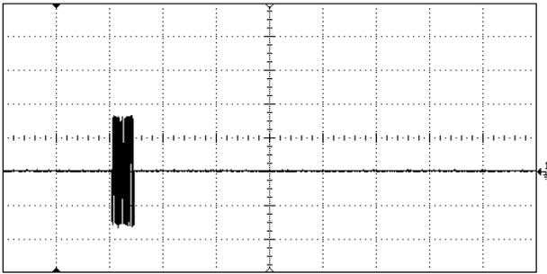
Figure 16: Experimental results. Over voltage protection operation under no load conditions. Gate voltage of  $Q_2$ . Horizontal scale: 20ms/div.
