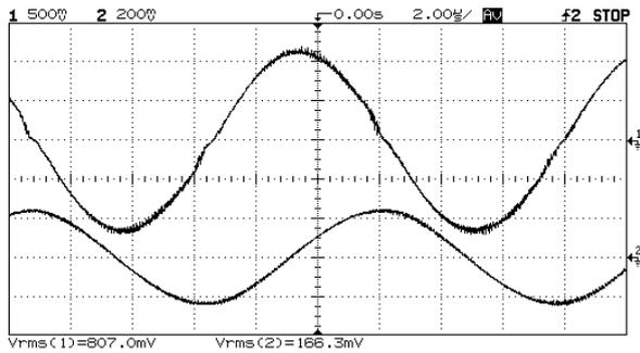
Figure 12. Experimental results, constant current when loaded by 1600Ω : top:  $I_{out}$  (0.2A/div); bottom  $I_{lamp}$  (0.2A/div); Horizontal scale: 2μS/div
