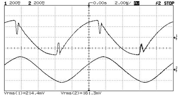
Figure 9. Experimental results, constant current when loaded by 300 $\Omega$  : top:  $I_{out}$  (0.2A/div); bottom  $I_{lamp}$  (0.2A/div); Horizontal scale: 2 $\mu$ S/div
