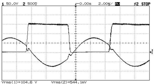
Fig. 15. Experimental results, ZVS operation when loaded by 1000Ω : top: drain voltage of  $Q_2$  (50V/div); bottom  $I_{out}$  (0.5A/div); Horizontal scale: 2μS/div
