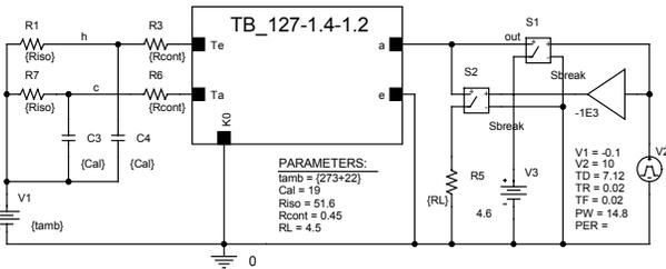
Fig. 7. PSPICE model for simulating the experiment.  $R_{iso}$  is a thermal resistance of the thermal insulation,  $C_{al}$  – thermal capacity of the aluminum plates.  $R_{cont}$  – thermal resistance of the thermal contact between TEM and the plate.
