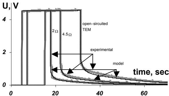
Fig. 8. Measured and simulated TEM voltage when used as a TEG for different loads.
