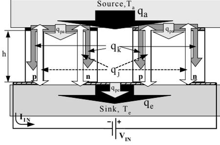
Fig. 1. Energy equilibrium for thermoelectric cooler.
