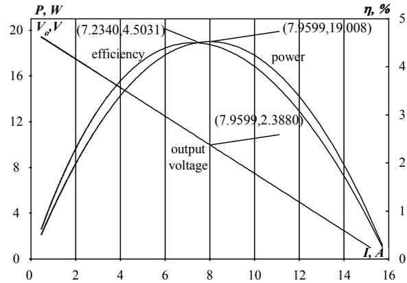
Fig. 4. DC-sweep simulation of performance of the Thermoelectric Generator HZ-20 made by Hi-Z Technology, Inc.
