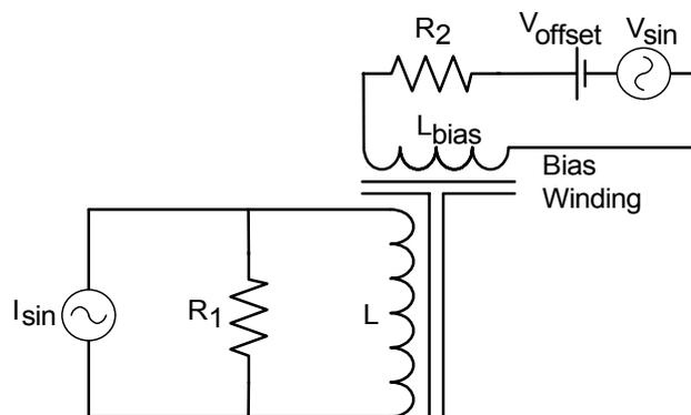
Figure 2. Parametric Modulation circuit.
