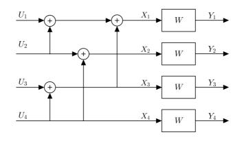
For items (a) to (c), assume that the bits  $U_1$  and  $U_2$  are frozen to 0, while  $U_3$  and  $U_4$  are used for message bits.
