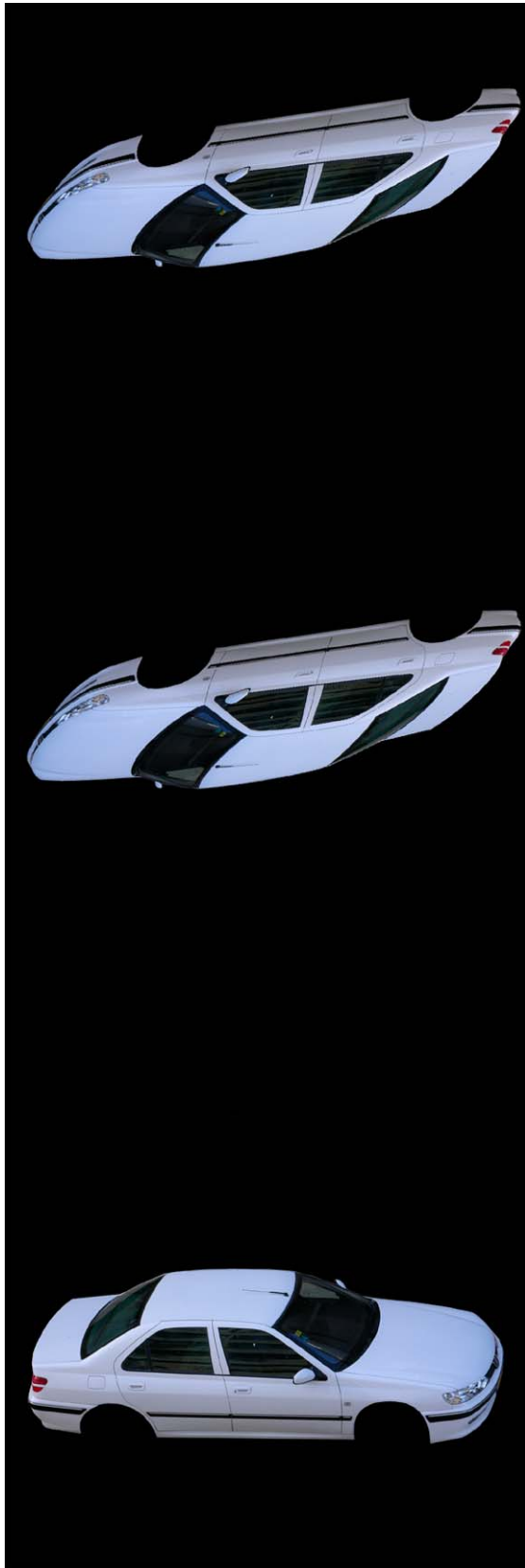
Fig. 1 From bottom to top : Template; Estimated deformed object obtained by applying the deformation estimated from the observation to the template; Observation on the deformed object
