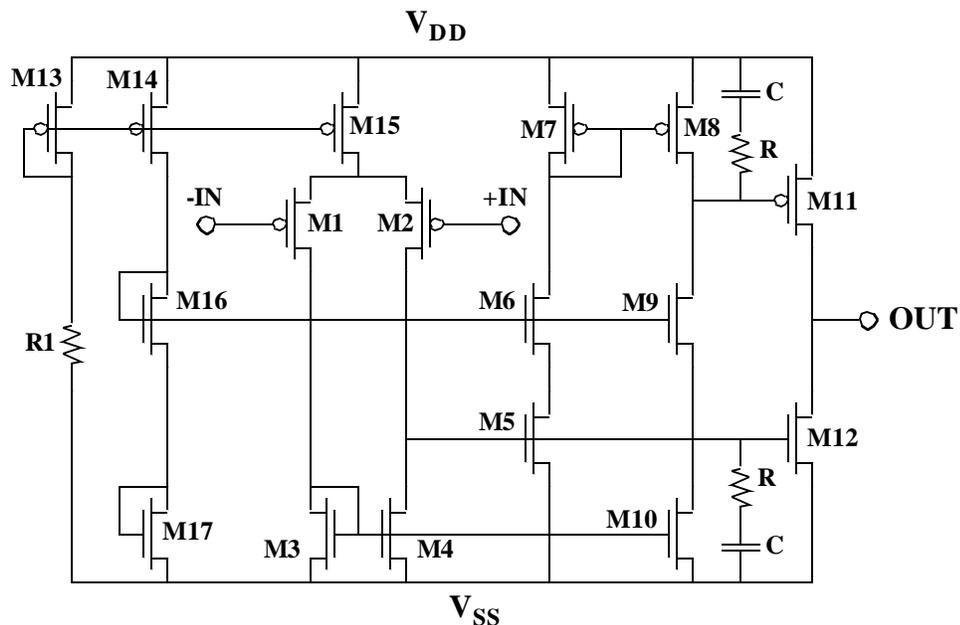
Here, M13-M15 establish the bias currents for the amplifier, while the stack of M16 and M17 provide a bias voltage for common-gate cascode devices M6 and M9.
