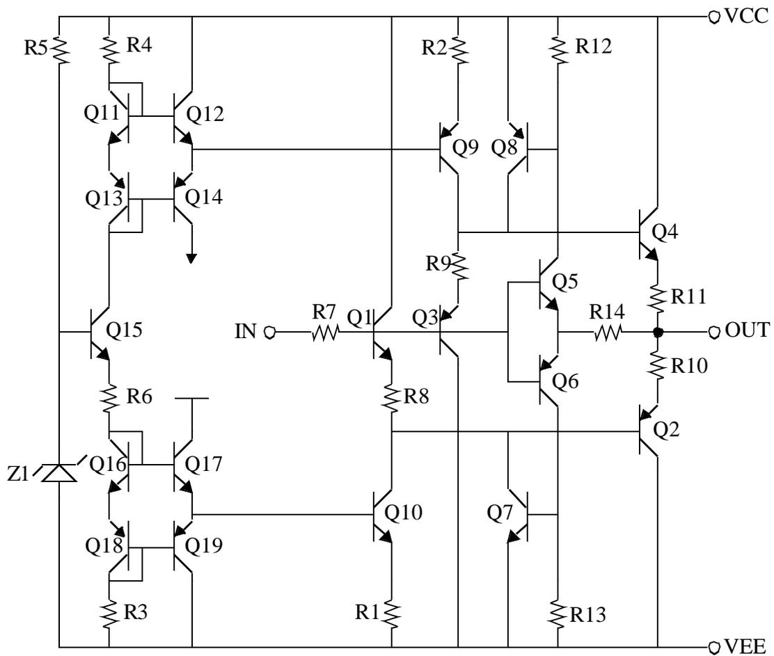
We see, then, that the HA-5033 contains the electronic equivalent of a turbocharger, where the part consumes a relatively small amount of power under most conditions, but is capable of temporary boosts in performance as needed.
