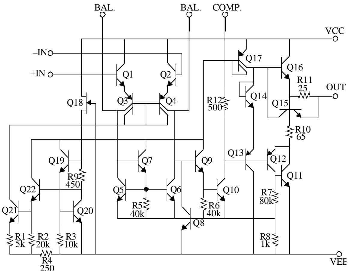
Another change, enabled by process improvements that produce higher PNP  $\beta$ , is simplified biasing of Q3/Q4 and Q17. The multiple collectors may be thought of as a shorthand notation for mirrors, where the current ratios are set by collector area ratios. Finally Q18,
