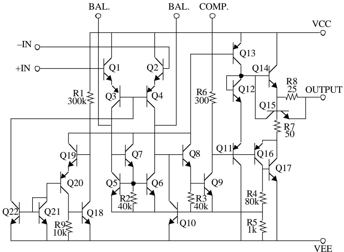
To improve input common-mode range, Widlar had to develop a more satisfactory solution to the level shift problem. A battery-based shifter, after all, more than simply re-centers the common-mode level; it also necessarily subtracts from it. The traditional alternative to a battery is simply to alternate NPN- and PNP-based stages, where the downward common mode shift of the latter compensates for the upward shift of the former.
