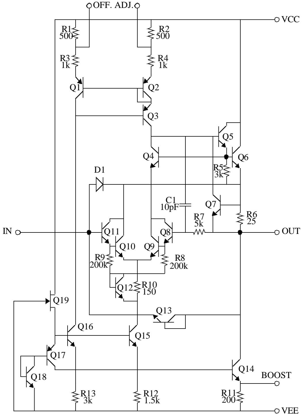
As one might expect, the LM110 is based on an op-amp, but with the feedback connection already provided internally. The op-amp at the heart of the LM110 is a single stage current-source loaded common emitter differential amplifier. The differential pair, Q8-Q11 consists of Darlington-connected devices to reduce base current (which, as always, must be supplied by the external source that drives the amplifier input). The actual input transis-
