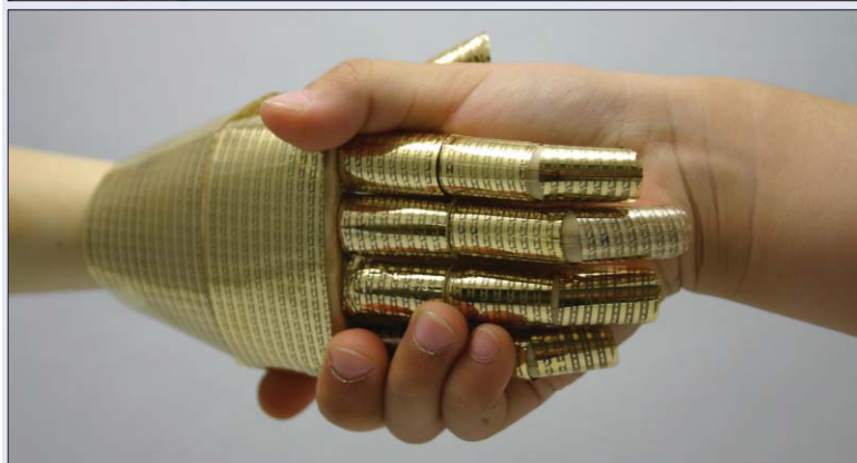
An electronic book made of organic transistors constructed from polymer thin-film transistors (top). A flexible sheet containing pentacene transistors, intended to create a layer of “skin” sensitive to pressure, is wrapped around a robot’s hand to give it the ability to “feel” (bottom).
