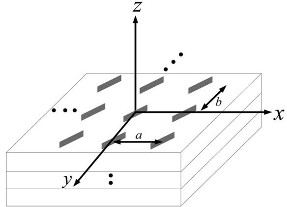
Fig. 1. Periodic structure on a general planar stratified structure.
