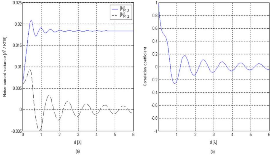
Fig. 2. Noise coupling between two unloaded  $\lambda/2$  dipole antennas versus the inter-element spacing,  $d$ . (a) Self noise current variance,  $[N_I]_{1,1}$  and mutual noise current covariance,  $[N_I]_{1,2}$ . (b) Noise current correlation coefficient,  $[C_I]_{1,2}$ .
