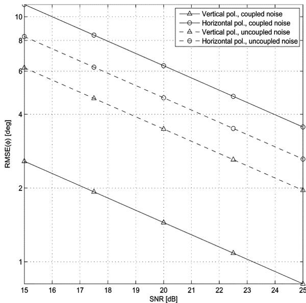
Fig. 5. CRLB curves for DOA estimation with incident signals of vertical and horizontal polarizations, with and without noise coupling, using the TLV antenna array.
