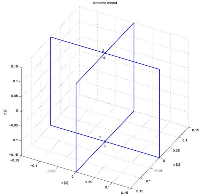
Fig. 3. TLV wire-antenna array with port locations.
