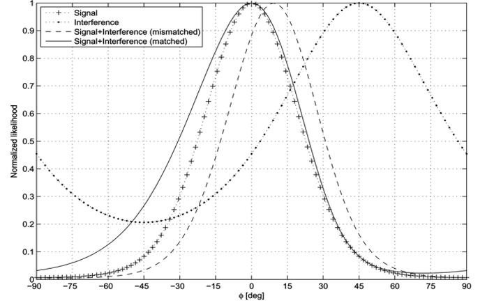
Fig. 6. The likelihood function for source localization: 1) signal without interference noise effect, 2) interference noise only, 3) signal with interference noise (mismatched model), and 4) signal with interference noise (matched model).
