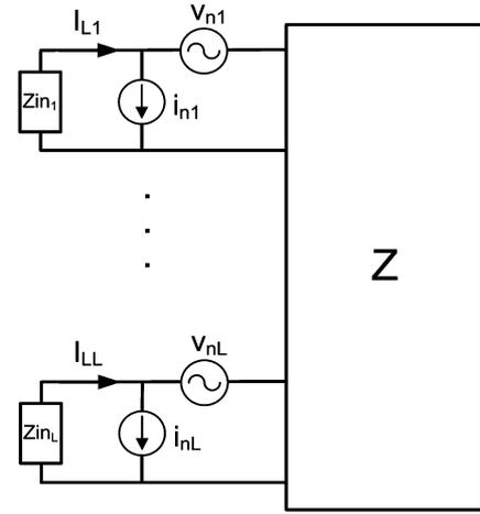
Fig. 1.  $L$ -port antenna array configuration loaded with LNAs.
