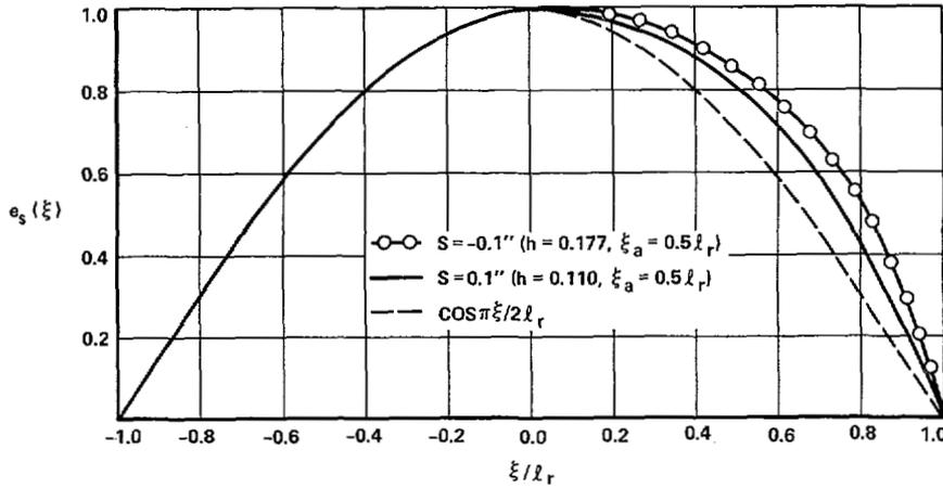
Fig. 5. Half-cosinusoid distribution and two perturbed distributions.
