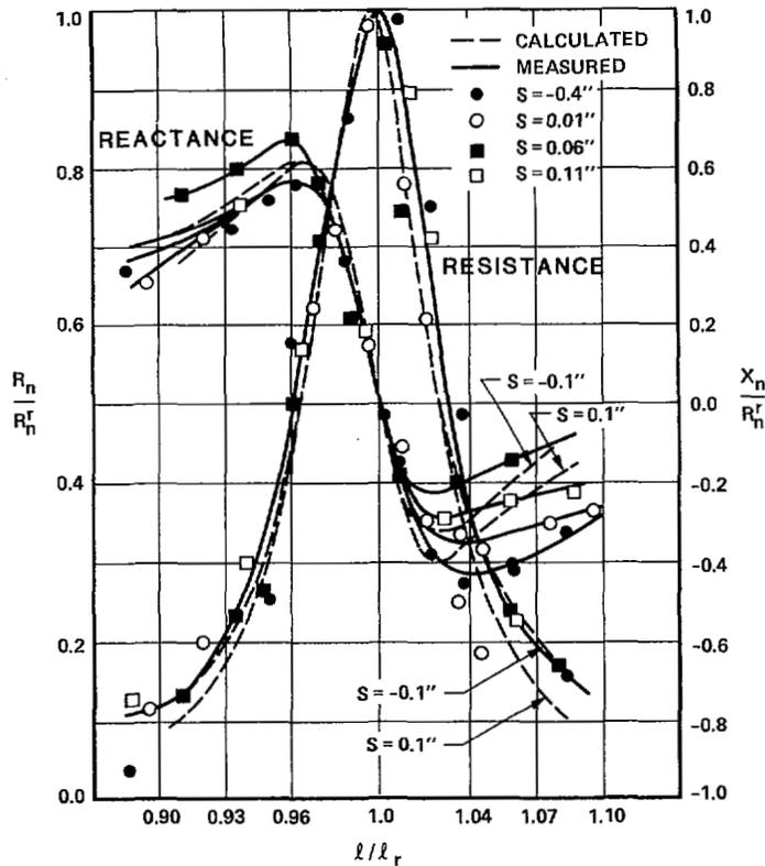
Fig. 4. Normalized resistance and reactance of the slot versus its normalized length.
