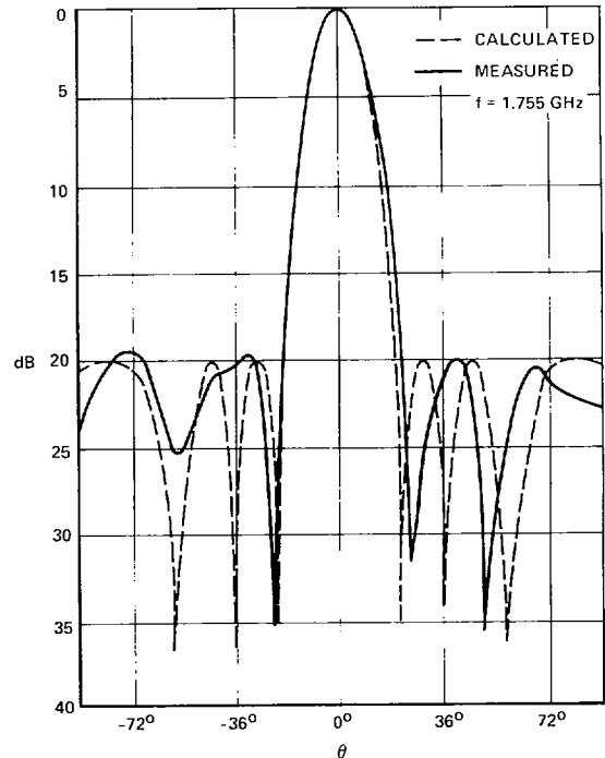
Fig. 6. Calculated and measured patterns for a six-element array,  $d = \lambda_g = 0.8 \lambda_0$ , with a 20 dB Dolph-Chebyshev distribution.
