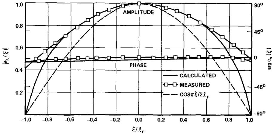
Fig. 2. Field distribution in a resonant slot ( $s = -0.1$  in).
