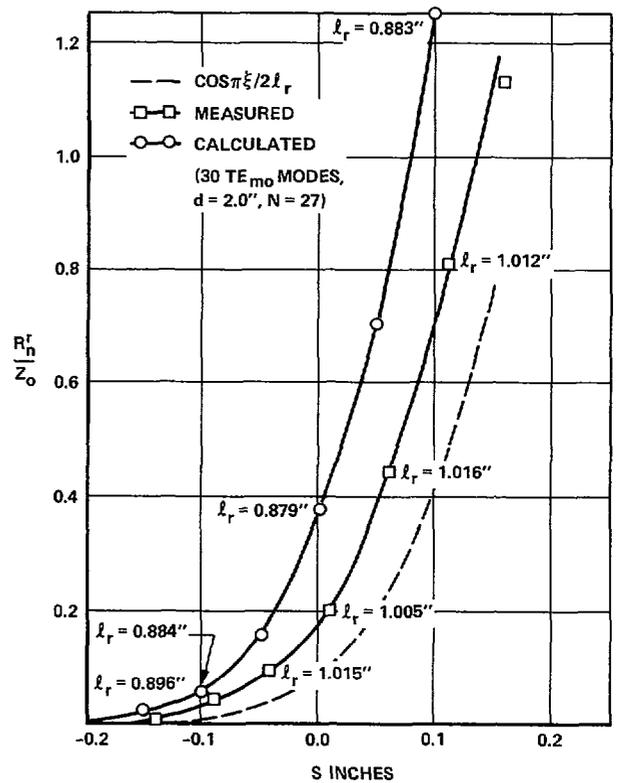
Fig. 3. Normalized resonant resistance of the slot versus the offset  $s$ .
