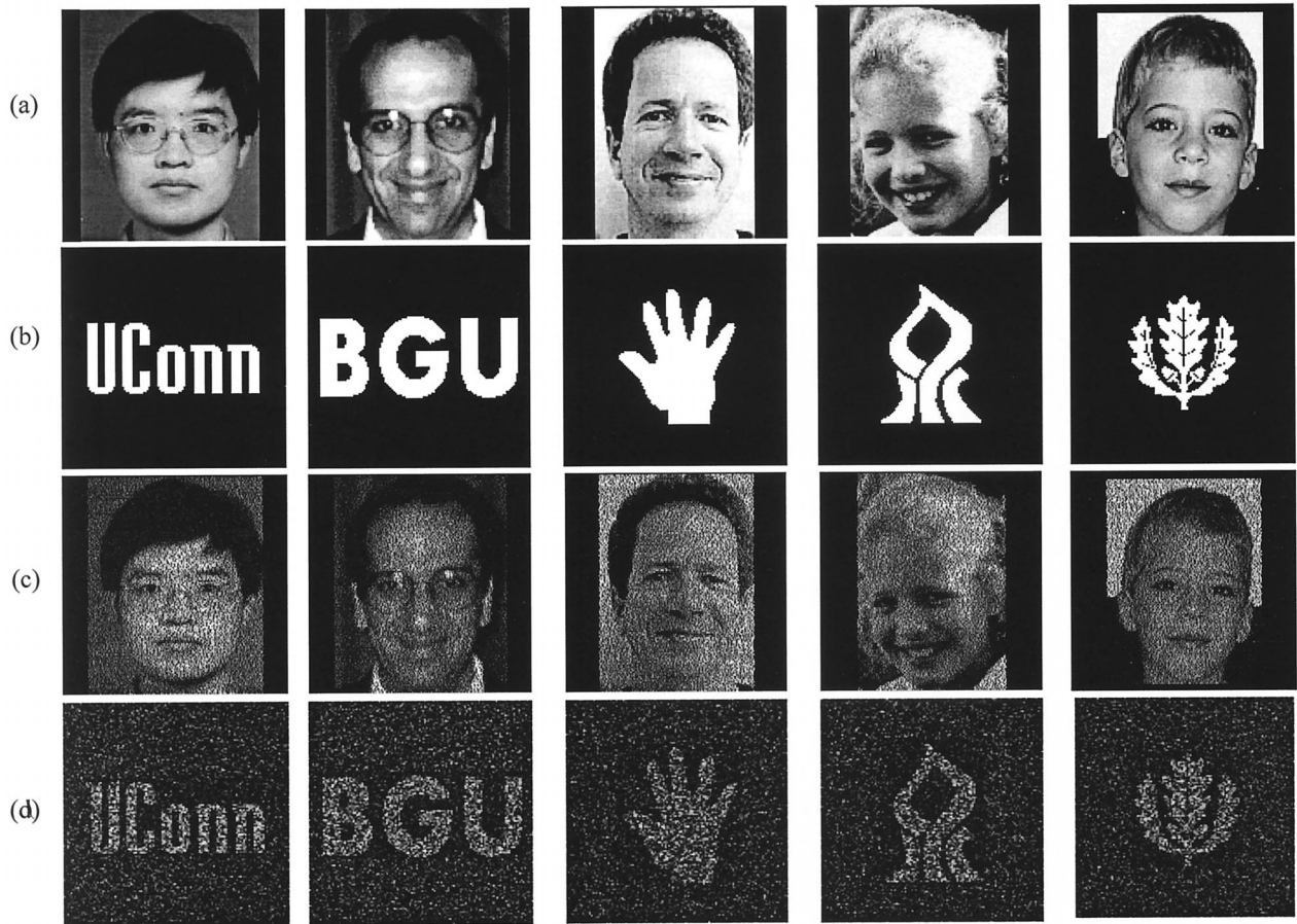
Fig. 5. (a) Original set of gray-tone pictures used as the visible images. (b) Original set of binary pictures used as the hidden images. (c) The resultant halftone images. (d) The hidden images revealed by the correlation between the set in (c) and the key function.
