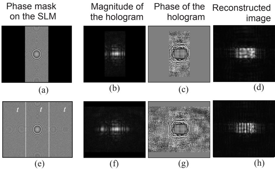
**Fig. 2.** Results of SAFE with the narrow aperture (Top) and with the synthetic aperture (Bottom).
