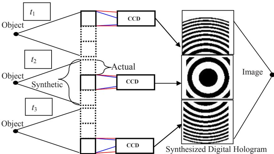
**Fig. 1.** Scheme of SAFE operating as synthetic aperture radar to achieve super-resolution
