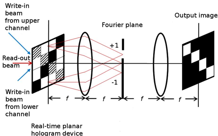
every two sequential pinholes to be equal to  $\frac{\lambda f}{sb}$ , where  $\lambda$  is the laser wavelength and  $f$  is the focal distance of the lenses in the channel. This gap limitation guaranties that the various duplications of the input matrix  $B$  are displayed on plane  $P_2$  adjusted to each other, without spaces between or overlaps among every two sequential duplicats.
