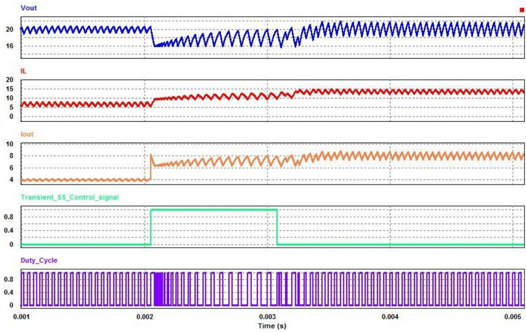
Simulation of minimal deviation control scheme on Boost converter using PSIM
