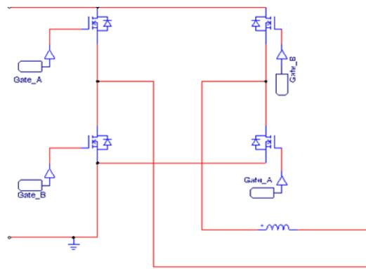
Fig. Second level simulation circuit (PSIM)
