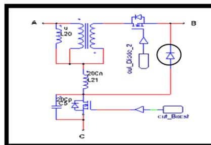
Fig. bypass diode (marked) in the first level circuit
