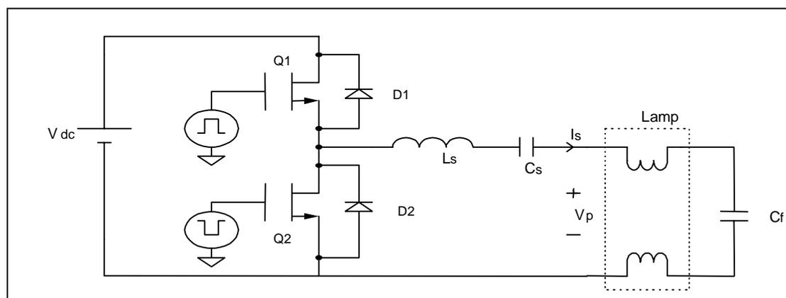
The series capacitor eliminates the DC current. The higher the frequency, the higher impedance of the inductor will decrease the current to the lamp. The lower the frequency, the lower impedance of the inductor will increase the current to the lamp.
