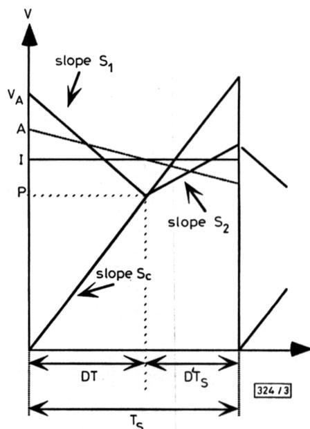
Fig. 3 Basic ACM waveforms
