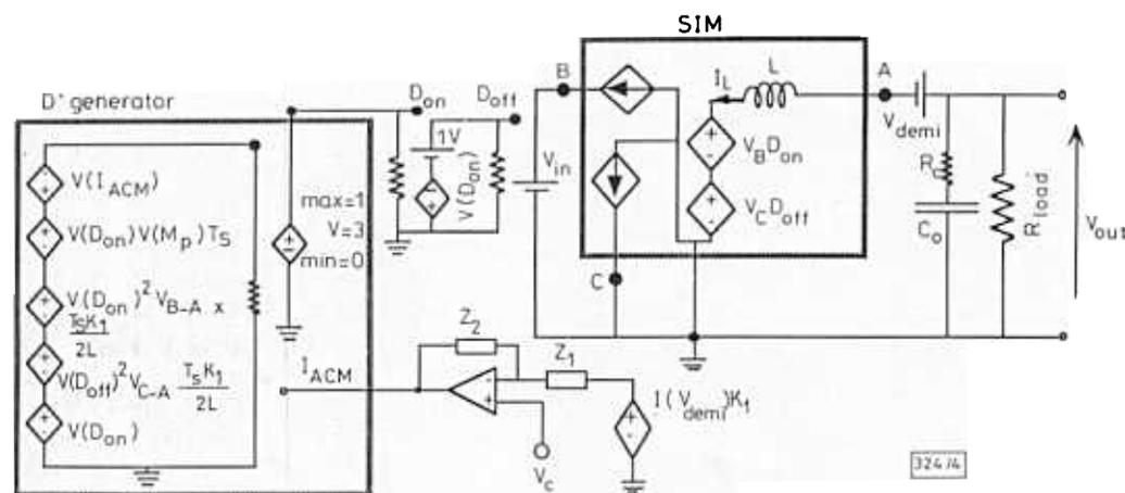
Fig. 4 SPICE compatible equivalent circuit of GCM model
