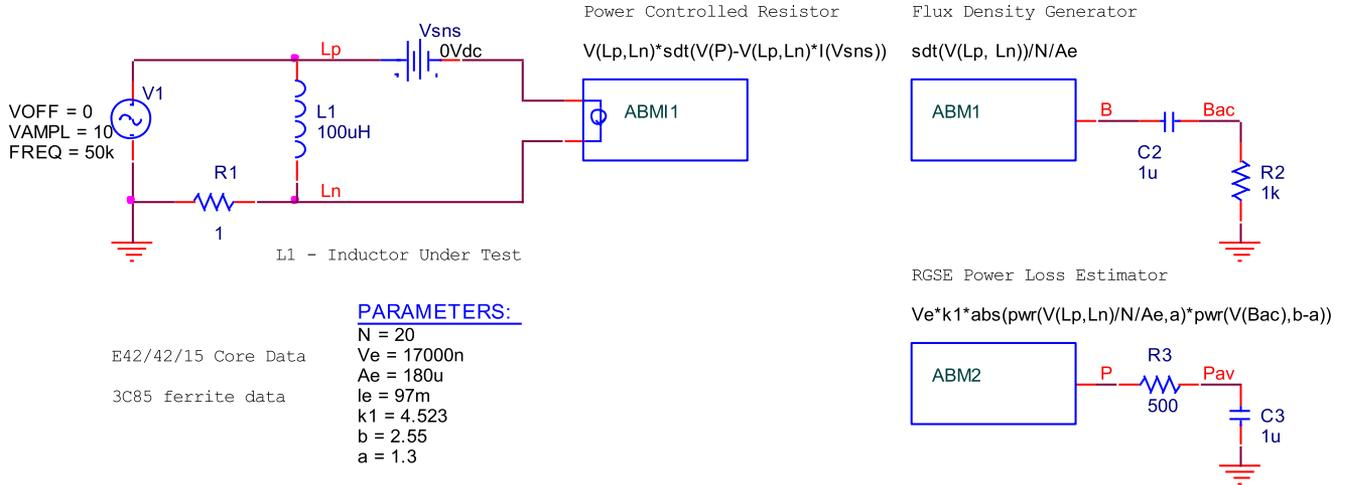
Fig. 2. Schematic diagram of RGSE-based SPICE core loss estimator of L1 inductor core loss under sinusoidal excitation.
