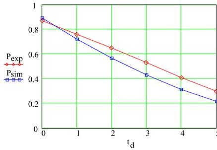
Fig. 9. Comparison of the simulated power loss ( $P_{sim}$ ) versus experimentally measured loss ( $P_{exp}$ ) [14] in the transformer core in a DAB as function of the zero voltage interval (time delay)  $t_d$ .
