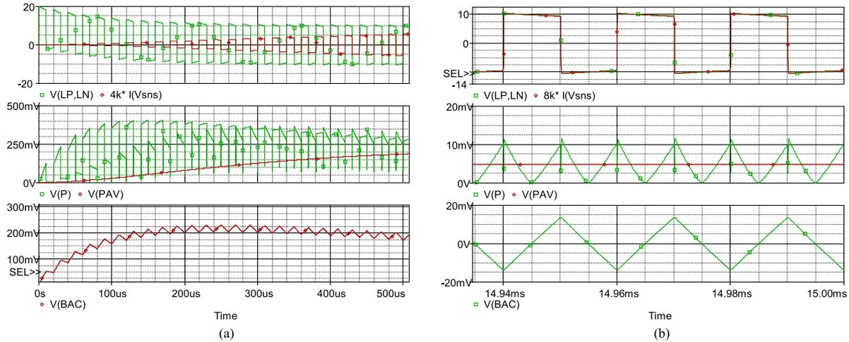
Fig. 5. (a) Typical simulation waveforms of RGSE power loss estimator under unipolar rectangular excitation: start-up transient; (b) steady-state. Upper screen- the inductor's voltage,  $V(LP, LN)$ , and the scaled PCR current,  $4k^* I(Vsns)$ ; middle screen- the instantaneous core power loss,  $V(P)$ , and the average core power loss,  $V(PAV)$ ; bottom screen- the ac flux density,  $V(BAC)$ .
