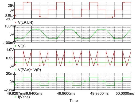
Fig. 8. Typical RGSE simulation waveforms of a DAB. Upper screen - inductor's voltage,  $V(LP, LN)$ ; middle screen- core flux density,  $V(B)$ ; bottom screen- the instantaneous core power loss,  $V(P)$ , and the average core power loss,  $V(PAV)$ .
