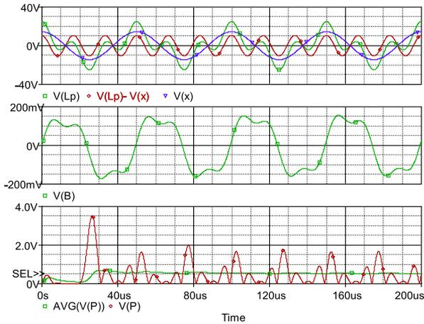
Fig. 6. Typical RGSE simulation waveforms under harmonically related sinusoidal excitation ( $C = 0.2$ ). Upper screen – the low frequency source signal,  $V(x)$ , the triple harmonic source signal,  $V(Lp)-V(x)$ , and the resulting inductor's voltage,  $V(Lp)$ ; middle screen- the core flux density,  $V(B)$ ; bottom screen- the instantaneous core power loss,  $V(P)$ , and the average core power loss,  $AVG(V(P))$ .
