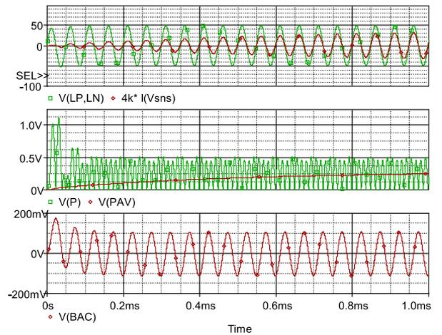
Fig. 3. Typical simulation waveforms of RGSE core power loss estimator under pure sinusoidal excitation. Upper screen—the inductor's voltage,  $V(LP, LN)$ , and the scaled PCR current,  $4k * I(Vsns)$ ; middle screen— the instantaneous core power loss,  $V(P)$ , and the average core power loss,  $V(PAV)$ ; bottom screen—the ac flux density,  $V(BAC)$ .
