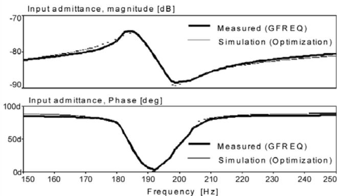
Fig. 3. Comparison between measured and model calculated admittances. Estimated parameters:  $C_{in}=64.36nF$ ,  $L_r=106.7H$ ,  $C_r=6.78nF$ ,  $R_m=6.75K\Omega$ .
