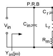
Fig. 1. Equivalent circuit of the Piezoelectric Resonator Blade (PRB)
