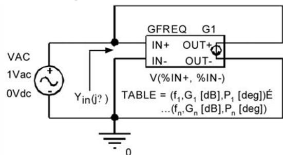
Fig. 2. Behavioral model of the resonator. The table of the GFREQ dependent source lists the measured admittance (magnitude and phase) over the measured frequency range
