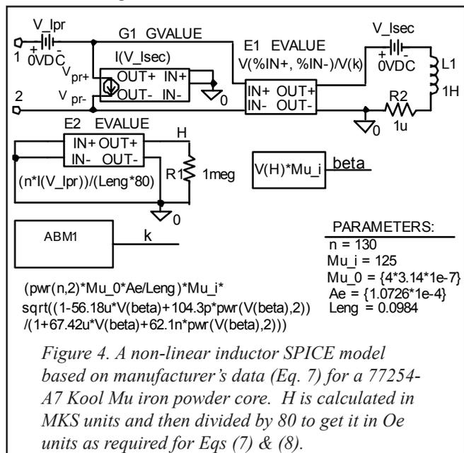
Figure 4. A non-linear inductor SPICE model based on manufacturer's data (Eq. 7) for a 77254-A7 Kool Mu iron powder core.  $H$  is calculated in MKS units and then divided by 80 to get it in Oe units as required for Eqs (7) & (8).
