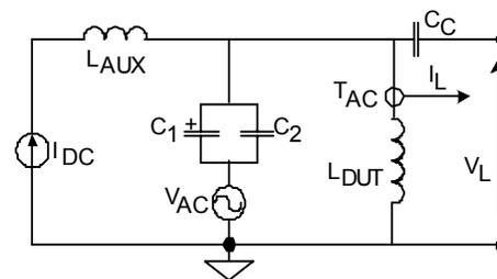
Figure 2. Experimental setup for measuring the small signal impedance of a dc biased inductor.
