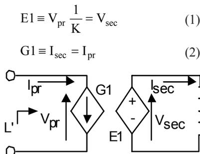
Figure 1. A non-linear inductor model built by reflecting a linear inductor via a non-linear 'transformer.'
