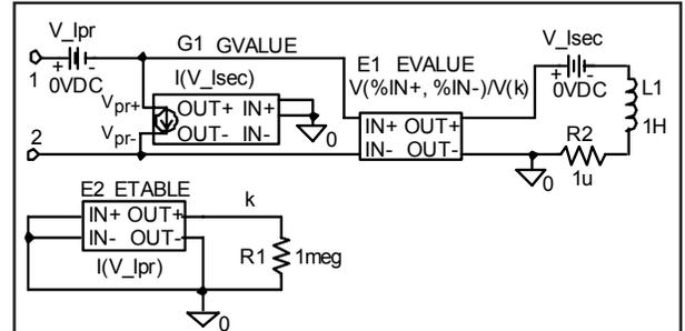
Figure 3. A non-linear inductor SPICE model based on measured inductance values. The table of the ETABLE dependent source lists the measured inductance as a function of dc current.
