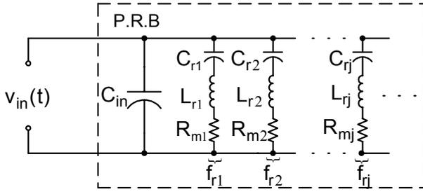
Figure 3. Equivalent circuit model of the PRB element.  $C_{in}$  is the dielectric capacitance of the input electrodes.
