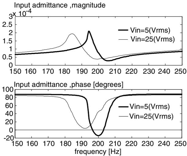
Figure 6. Input admittance of experimental PRB for two excitation voltages.
