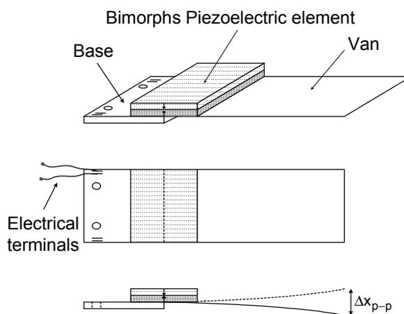
Figure 1. The piezoelectric resonant blade element.
