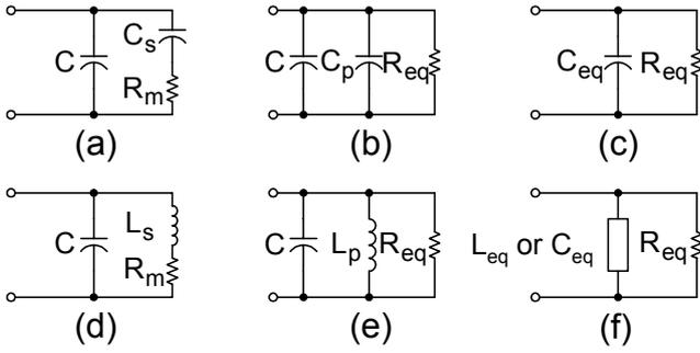
Figure 7. Equivalent circuits of the PRB at various operating frequency ranges. (a), (b), (c) are equivalent circuits for  $f < f_r$ ; (d), (e), (f) are equivalent circuits for  $f > f_r$ . In last frequency range the input admittance could be capacitive or inductive.
