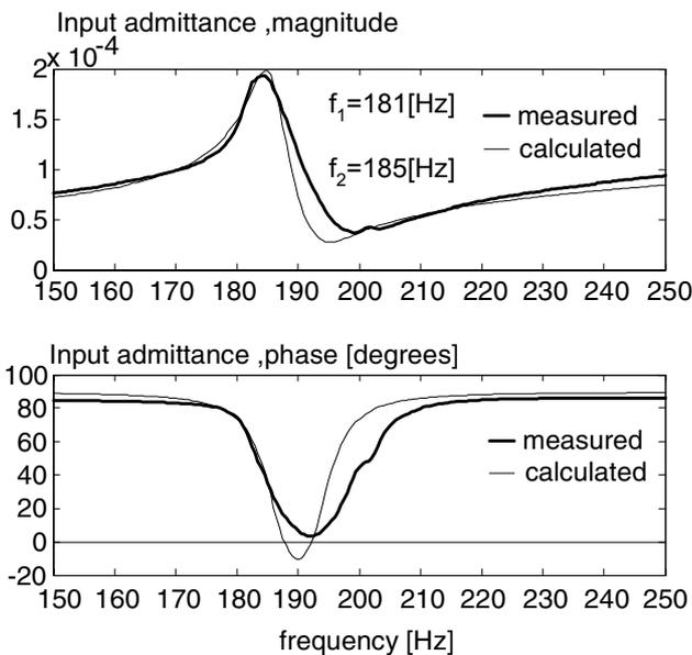
Figure 12. Comparison between measured and model calculated admittances. Model parameters extraction by Method A;  $C$  was calculated by eq. (3).  $f_1$  and  $f_2$  are two arbitrary frequencies in the range  $f < f_r$ . Estimated parameters:  $C=59.961\text{nF}$ ,  $L_r=134.8\text{H}$ ,  $C_r=5.4363\text{nF}$ ,  $R_m=5773\Omega$ ,  $f_r=185.92\text{Hz}$ .
