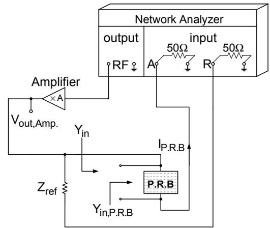
Figure 9. Network analyzer measurements setup.
