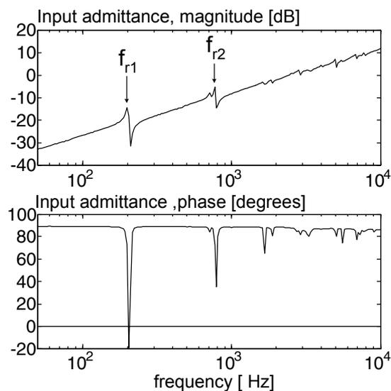
Figure 2. Input admittance of the PRB element. The series resonant frequencies  $f_{r1}$ ,  $f_{r2}$  correspond to first and second vibration modes.
