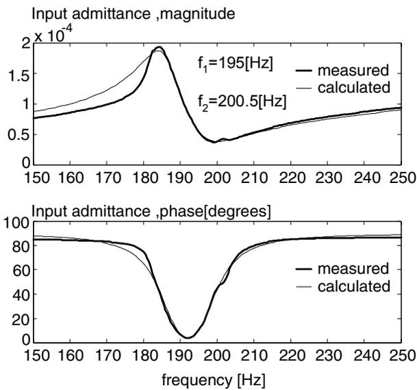
Figure 11. Comparison between measured and model calculated admittances. Model parameters extraction by Method C. Fitting range: 187.5Hz to 204.5Hz ( $f > f_i$ ). Estimated parameters:  $C=67.8\text{nF}$ ,  $L_r=84.551\text{H}$ ,  $C_r=8.6184\text{nF}$ ,  $R_m=6508\Omega$ ,  $f_r=186.443\text{Hz}$ .
