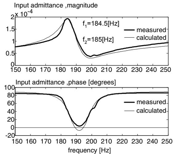
Figure 10. Comparison between measured and model calculated admittances. Model parameters extraction by Method C. Fitting range: 181Hz to 189Hz ( $f < f_r$ ).  $f_1$  and  $f_2$  were found by the MATLAB least square fitting algorithm as to provide the best fit. Estimated parameters:  $C=60.7\text{nF}$ ,  $L_r=95.481\text{H}$ ,  $C_i=7.6458\text{nF}$ ,  $R_m=5987.6\Omega$ ,  $f_r=186.27\text{Hz}$ .
