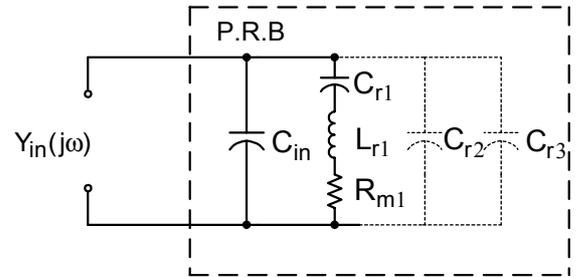
Figure 4. Approximate electrical circuit model near the first resonant frequency. Dashed branches corresponding to the strong capacitive influence of higher resonance harmonics.
