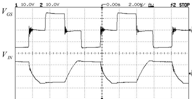
Fig. 8. Experimental voltage waveforms of the half-bridge inductor-less PT inverter:  $V_{GS}$  (upper plot),  $V_{IN}$  (lower plot). Operating frequency  $f=120kHz$ , load resistance  $R_L=130$  Ohm. Data is for T1-2, Transoner<sup>R</sup>) [10].
