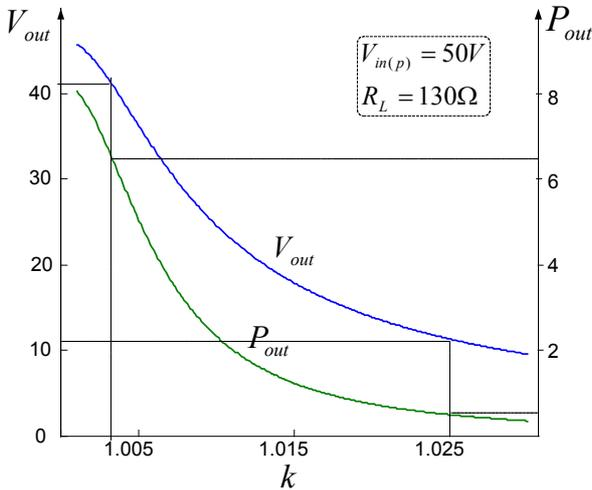
Fig. 7. The peak output voltage  $V_{out(p)}$  and the output power  $P_{out}$  as a function of the normalized frequency factor  $k$  for peak input voltage  $V_{in(p)} = 50V$  and load resistance  $R_L = 130\Omega$ . Data is for T1-2, Transoner<sup>R</sup>) [10].
