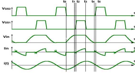
Fig. 2. The steady-state current and voltage waveforms of the ZVS PT inverter.
