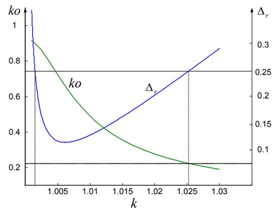
Fig. 5. Voltage transfer function  $ko$  and the normalized charging time  $\Delta_r$  as a function of the normalized frequency factor  $k$  for normalized load factor  $Q=0.15$  ( $R_L = 130\Omega$ ). The PT under the calculations is (T1-2, Transoner<sup>R</sup>) [10].
