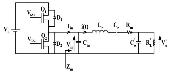
Fig. 1. Equivalent circuit of a half bridge inverter driving a PT around the resonant frequency.
