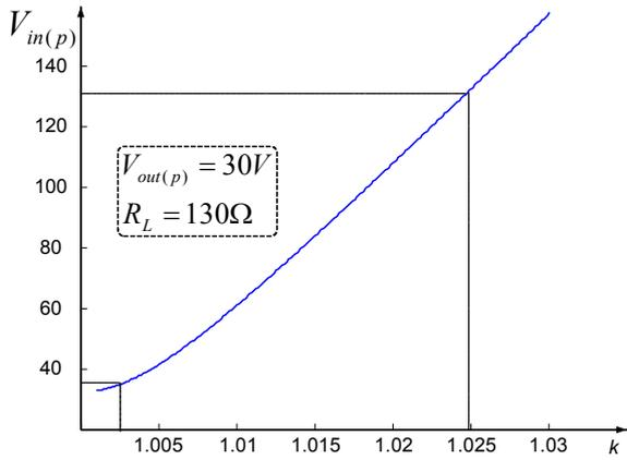
Fig. 6. Peak input voltage  $V_{in(p)}$  as a function of the normalized frequency factor  $k$  for the constant output peak voltage  $V_{out(p)} = 30V$  and the load resistance  $R_L = 130\Omega$ . Data is for T1-2, Transoner<sup>R</sup>) [10].
