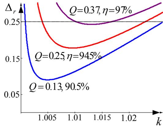
Fig. 3. Normalized charging time as a function of the normalized frequency factor  $k$  for different normalized load factors  $Q$  in the range  $Q=0.13$  to  $Q=0.37$ . Data is for T1-2, Transoner<sup>R</sup> [10].
