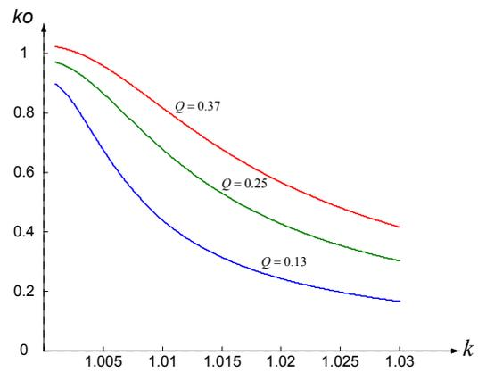
Fig. 4. Voltage transfer function  $ko$  as a function of the normalized frequency factor  $k$  for different normalized load factors  $Q$  in the range of  $Q=0.13$  to  $Q=0.37$ . The PT under the calculations is (T1-2, Transoner<sup>R</sup>) [10].
