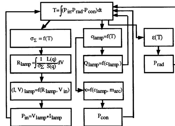
Fig.2. Solution structure of lamp state equation.
