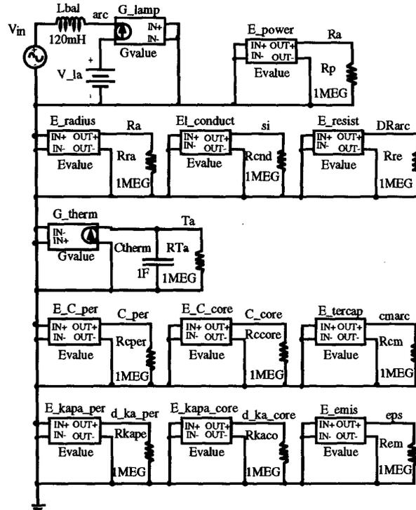
Fig. 4. SPICE model. See text for definitions of dependent voltage sources (EVALUE) and current source (GVALUE)
