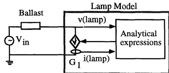
Fig.1. The proposed SPICE compatible model of an HID lamp.  $G_1$  is a behavioral dependent current source.
