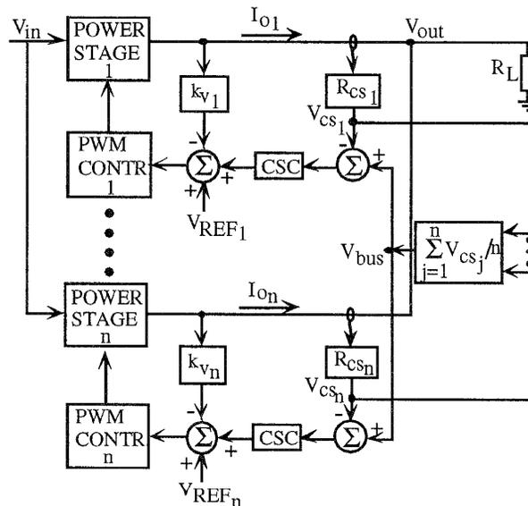
Fig. 1 Block diagram of  $n$  paralleled converters with Average Current Sharing (ACS).
