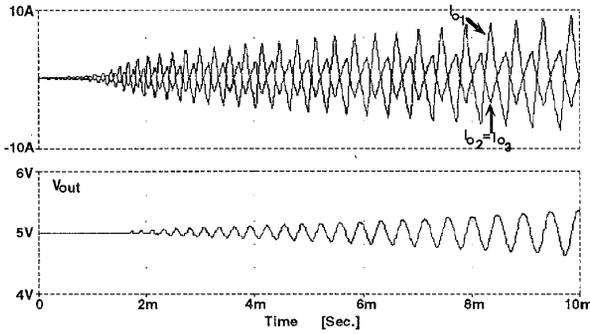
Fig. 12. Transient simulations of output currents and output voltage of three identical paralleled modules, with  $R_{f2}=0$ , when the pulse excitation is injected into the first module.
