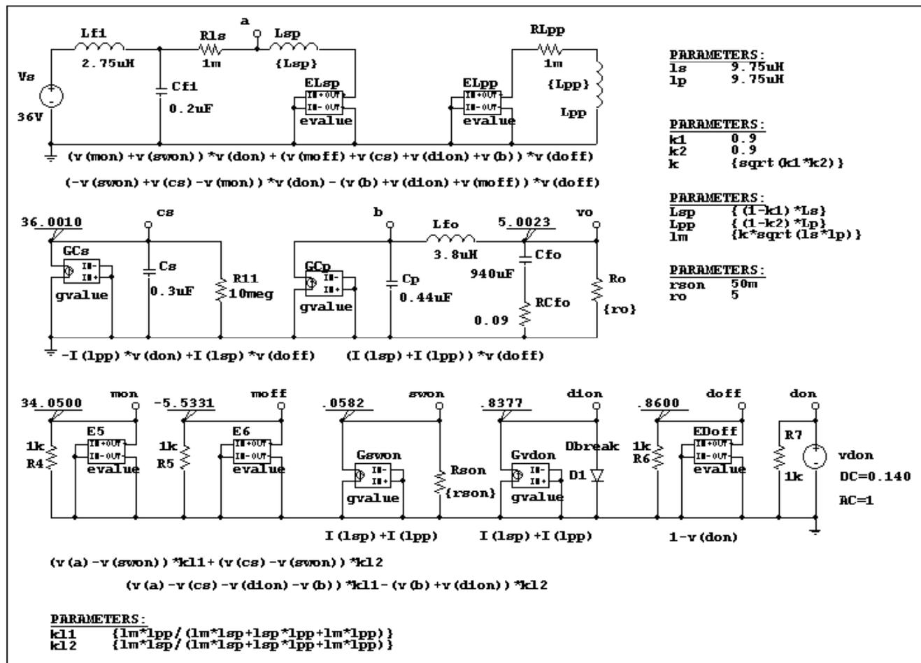
Fig. 8. 'Schematics' (MicroSim Inc.) diagram of the SEPIC average model for open loop simulations.
