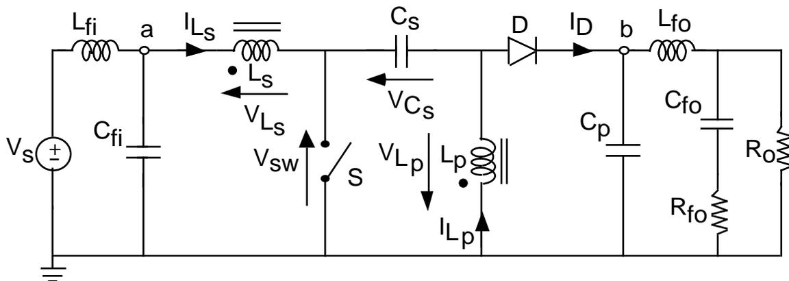
Fig. 1 DC to DC SEPIC converter with coupled inductors ( $L_S$  and  $L_P$ ), including input and output filters.
