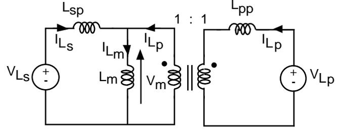
Fig. 3 The coupled inductors model with voltage sources representing the capacitors voltages.
