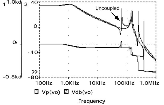
Fig. 6 AC small signal characteristics of SEPIC topology with coupled ( $k_1=k_2=0.9$ ) and uncoupled inductors. Operating point:  $D_{on}=0.14$ ,  $R_o=5$ .
