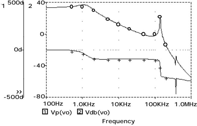
Fig. 5 AC small signal control-to-output  $\left[ \frac{V_o}{V_{don}}(f) \right]$  response of SEPIC converter with coupled inductors. Cycle-by-cycle simulations (o for Magnitude[db], + for Phase[deg]), compared to average model simulations (continuous lines). Operating point:  $D_{on}=0.14$ ,  $R_o=5$ ,  $k_1=k_2=0.9$ .
