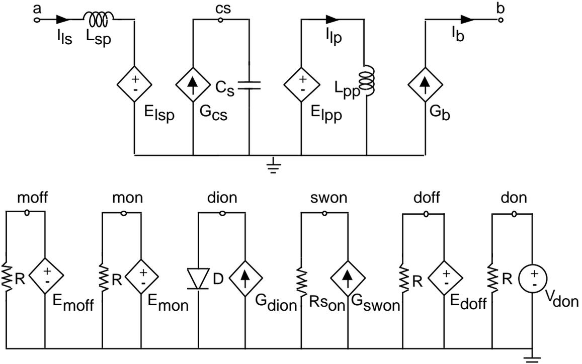
Fig. 4 Proposed behavioral average model for SEPIC converters with coupled inductors. Nodes names are marked by -o-.
