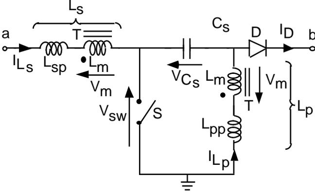
Fig. 2 Simplified diagram of the SEPIC topology with coupled inductors.
