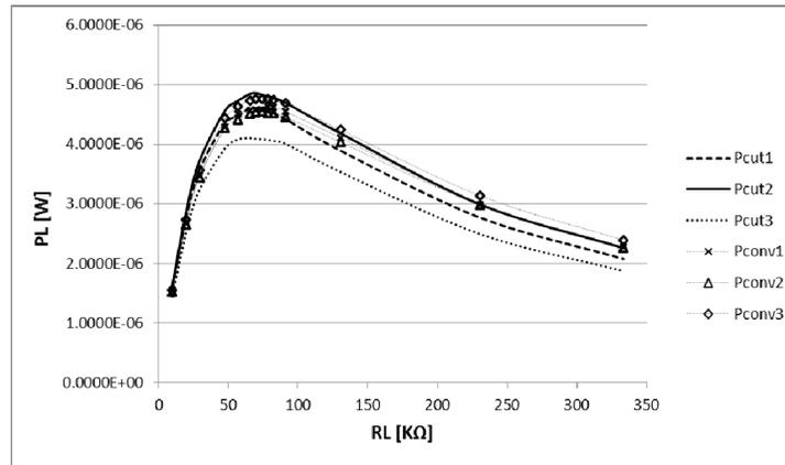
Fig. 4. Average output power vs. resistive load  $R_L$  for random excitation at a fixed input base acceleration of 0.145g (rms).  $P_{conv1}$ ,  $P_{conv2}$  and  $P_{conv3}$  are the results of a three-measurement set carried out with the conventional configuration.  $P_{cut1}$ ,  $P_{cut2}$  and  $P_{cut3}$  describe the three-measurement set results for the proposed generator. The experimental curves approach a maximum power point around  $R_L=74\text{K}\Omega$ .
