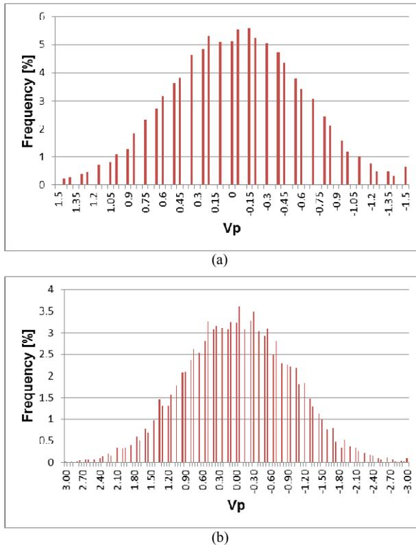
Fig. 6. Gaussian distribution of 50,000 time domain samples of the proposed generator output voltage,  $v_p$ , at an optimal load of  $74\text{K}\Omega$ . The standard deviation was found to be: (a)  $\sigma=0.5784\text{Vrms}$  @  $a_{\text{acc(rms)}}=0.145\text{g rms}$ , (b)  $\sigma=0.9378\text{Vrms}$  @  $a_{\text{acc(rms)}}=0.24\text{g rms}$ .
