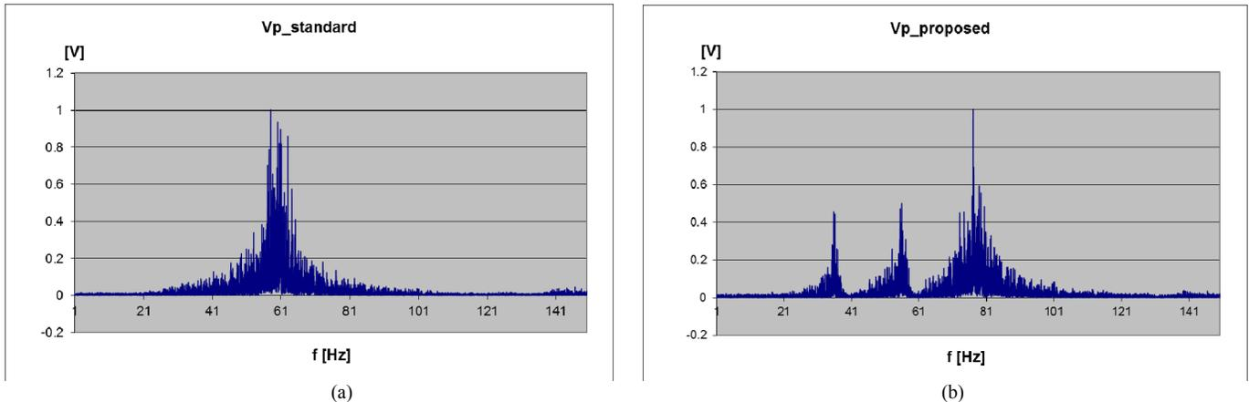
Fig. 5. Normalized FFT spectrum of the output voltage,  $v_p$ , under random excitation and with the same parameters as used in Fig. 3: (a) rectangular beam (b) proposed beam. Vertical units are volts [V] and horizontal units are Hertz [Hz].
