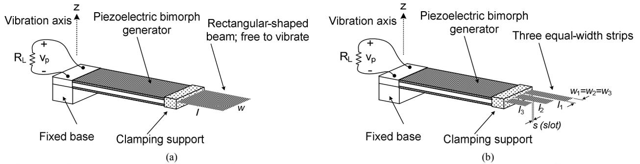
Fig. 1. Schematic of the piezoelectric generator with a cantilever beam: (a) rectangular beam, (b) proposed beam with three equal-width fingers.
