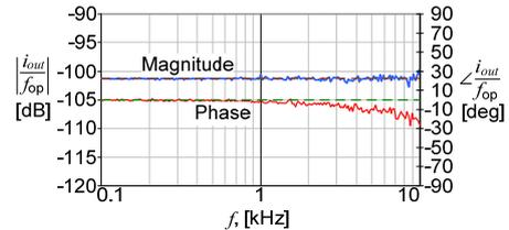
Fig. 10. Output-current to switching-frequency transfer function.
