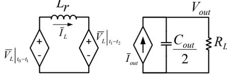
Fig. 5. Basic form of the behavioral model of proposed converter.
