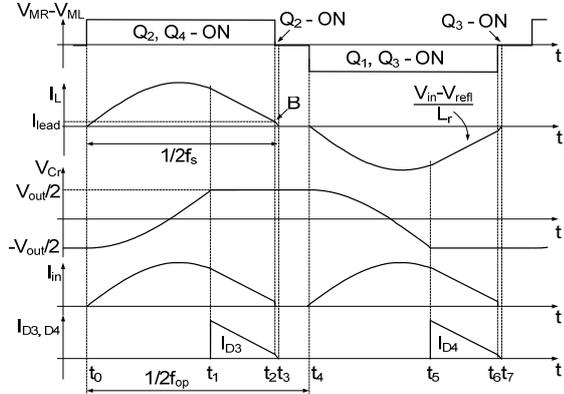
Fig. 3. Key waveforms of the proposed converter.
