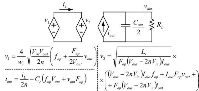
Fig. 7. Linearized average small signal model of the converter for small signal excitation in  $F_{op}$ , ( $f_{op}$ ).
