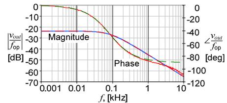
Fig. 9. Output voltage-to-switching frequency transfer function.
