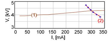
Fig. 4. Load characteristic of magnetron (1) and typical output characteristic of proposed resonant converter (2): solid line – calculated according to (7); dots – cycle-by-cycle simulation results.
