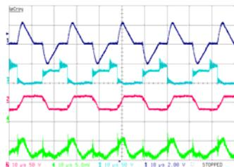
Fig. 11. Typical experimental results; loaded by magnetron. Upper trace: Inductor current 200A/div; Second trace from top:  $V_{MR}$  (Fig. 2) 50V/div; Third trace from top: Transformer primary voltage 100V/div; Lower trace: Microwave power 880W/div; Horizontal scale: 10us/div.
