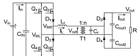
Fig. 2. Proposed topology with input diodes.
