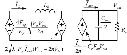
Fig. 6. Behavioral model of converter.
