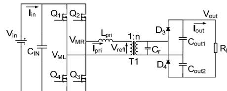
Fig. 1. Parallel resonant converter with output voltage doubler.
