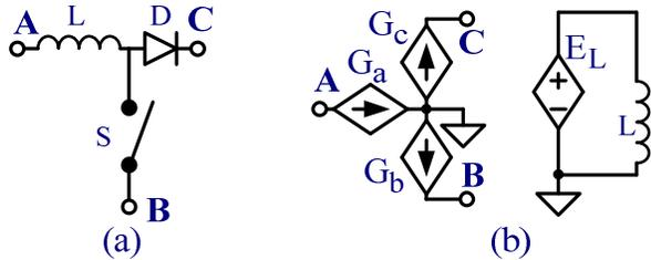
Figure 2. PWM Converters (a) Common block, (b) Generic switched inductor model - GSIM.
