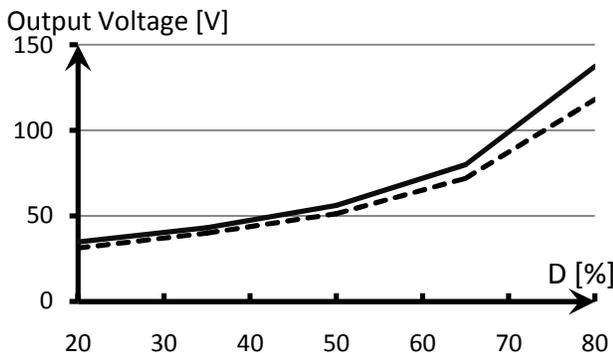
Figure 11. Boost SCCx3 model predicted output voltage as a function of duty cycle for  $V_m=10V$ : solid trace—capacitors' ESR=50mΩ; dashed trace—capacitors' ESR=1Ω.
