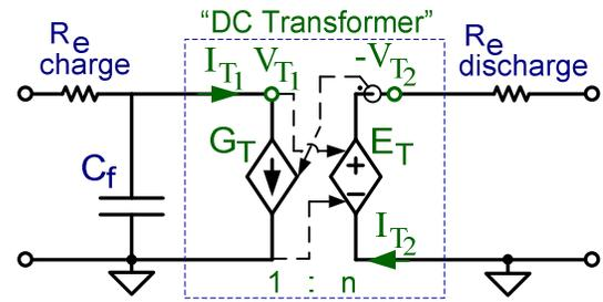
Figure 4. Average dynamic model of flying capacitor, including isolated charge transfer mechanism "DC Transformer".
