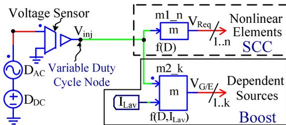
Figure 6. PSIM implementation of the average control model.
