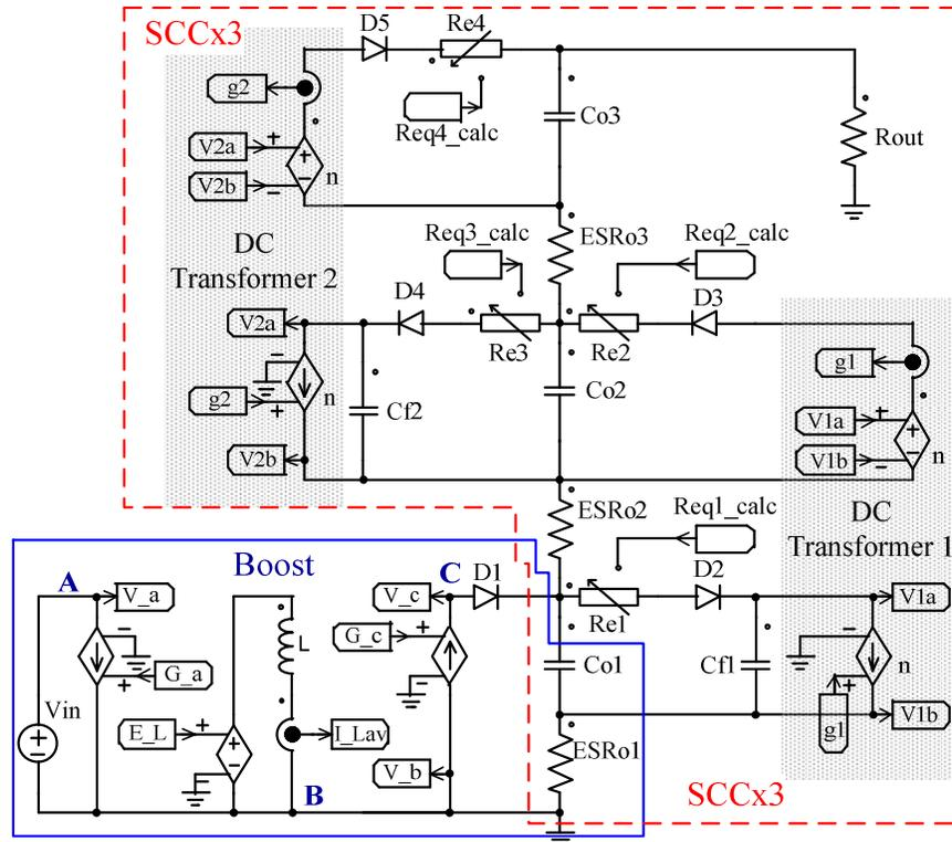
Figure 5. Average dynamic model of Boost SCCx3 system, including isolated charge transfer mechanism "DC Transformer", Implemented in PSIM.
