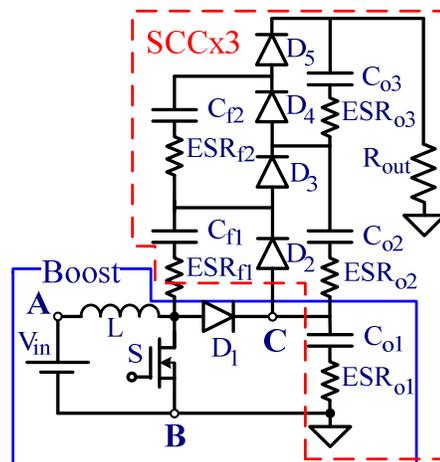
Figure 1. Hybrid Boost SCCx3 converter.
