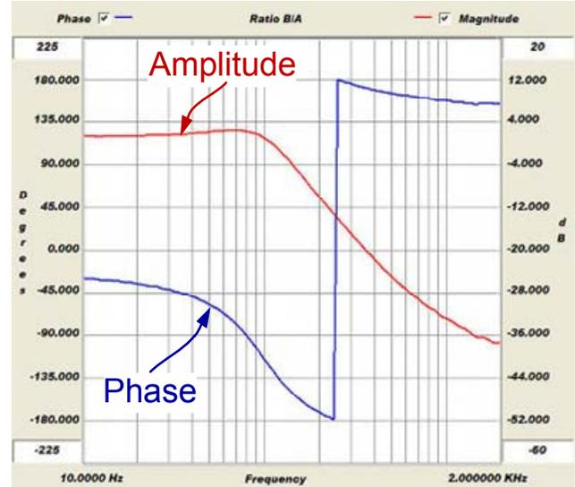
Figure 9. Experimental results of the control to output response of a Boost SCCx3 hybrid converter.
