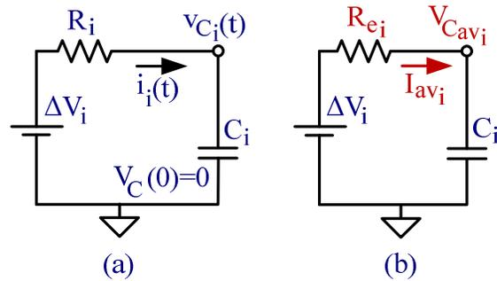
Figure 3. SCC subcircuit (a) Generic instantaneous charge/discharge circuit, (b) Generic average model.
