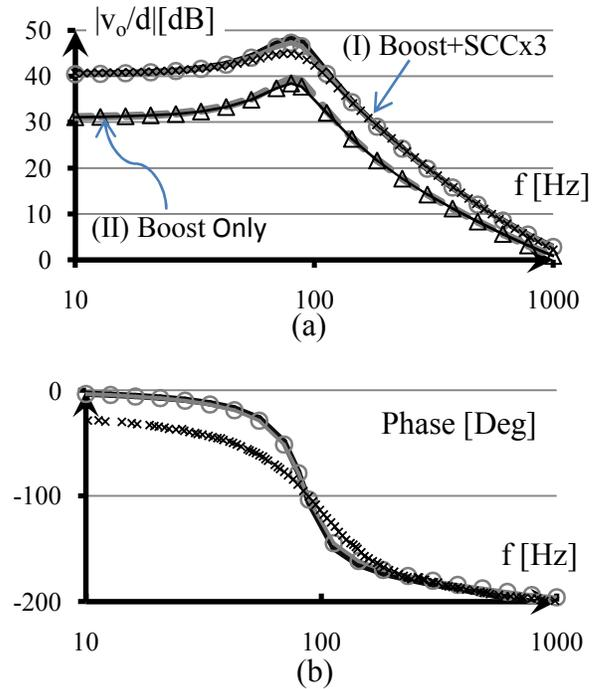
Figure 10. Control to output response of Boost only and hybrid converter: (a) Amplitude response; (I) Hybrid: experimental, cycle-by-cycle simulation, average model; (II) Boost only: cycle-by-cycle simulation, average model; (b) Phase response of hybrid converter: experimental, cycle-by-cycle simulation, average model.
