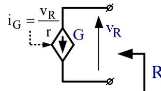
Figure 7. Emulation of a dependent resistor by a dependent current source,  $R = r$ .
