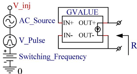
Figure 8. Implementation of a dependent equivalent resistance in PSpice.
