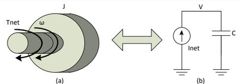
Figure 2. Mechanical to electronic analogy (a) mechanical system, (b) its electrical analog model.
