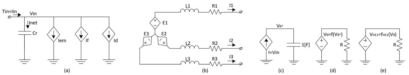
Figure 3. BLG modeling circuitry (a) electrical analog of mechanical shaft, (b) 3 phase stator, (c) shaft position detector, (d) shaft position to electrical angle converter, (e) Hall Effect sensor emulator.
