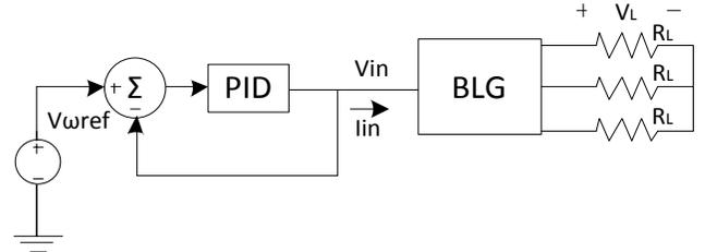
Figure 5. Simulation circuit for BLG model parameters extraction.
