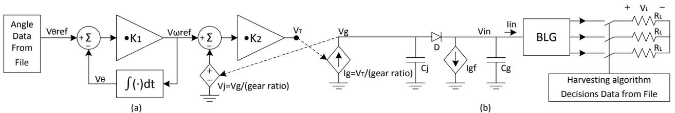
Figure 4. Model of the complete electro-mechanical system and its simulation control block, (a) simulation control block, (b) electro-mechanical system.
