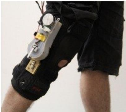
Figure 1. Knee energy harvesting - experimental prototype.
