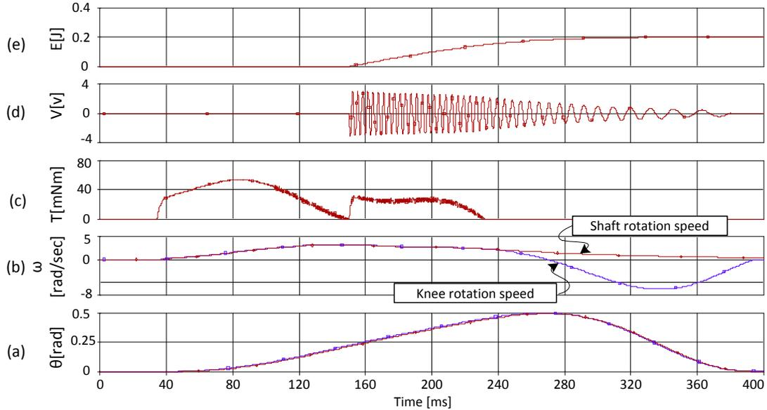
Figure 8. Example of simulation model prediction capabilities, (a) the input knee angle profile and the tracked emulated angle generated by the model (the traces are on top of each other), (b) knee and motor normalized rotation speed, (c) torque applied to the shaft, (d) load voltage of a single phase, (e) accumulated energy from a single phase.
