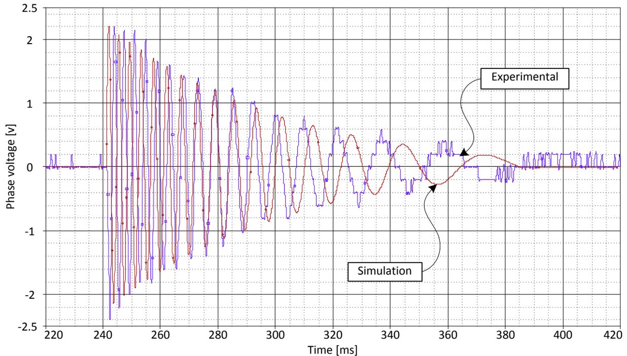
Figure 7. Simulation and experimental results for load voltage of a single phase during the harvesting
