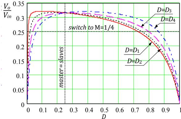
Fig. 4: The transfer functions  $V_o/V_{in}$  for different master duty cycles  $D=D_i$  selections and  $p=10$ .
