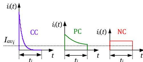
Fig. 3: Possible forms of the current through the equivalent capacitor  $C_i$  in topology  $i$ .
