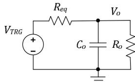
Fig. 1: The equivalent circuit of SCC
