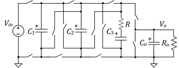
Fig. 5: The structure of the experimental setup circuit.
