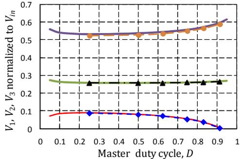
Fig. 8: The voltages across  $C_1, C_2, C_3$  normalized to  $V_{in}$  for  $M=3/8$  and  $D=D_1$ . Solid line: model prediction; Dashed line: experimental results.
