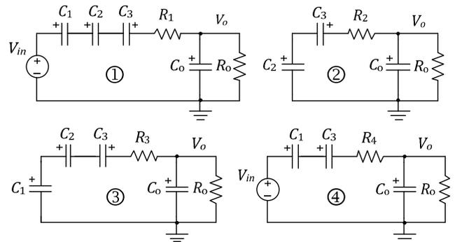
Fig. 2: Topologies of the SCC with the conversion ratio  $M = 3/8$ .
