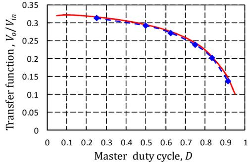
Fig. 7: The SCC regulation characteristics for  $M=3/8$  and  $D=D_1$ . Solid line: model prediction; Dashed line: experimental results.
