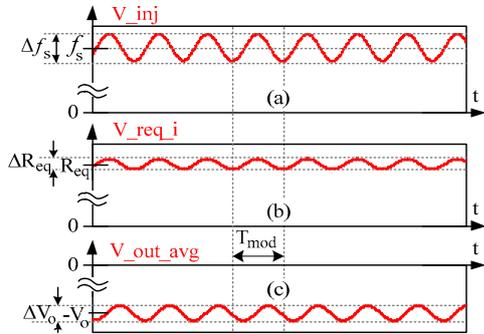
Figure 12. Typical waveforms along the generation chain of frequency dependent resistor (Fig. 10) in PSIM. (a) The voltage signal that represents the momentary frequency ( $V_{inj}$  Fig. 10); (b) The voltage signal that represents the equivalent resistance ( $V_{req\_i}$  Fig. 10a); (c) The resulting voltage modulation on the SCC output voltage.
