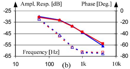
Figure 19. Small signal, control to output responses  $\{v_o/f_c(f)\}$  of the inverting 1:1 SCC, obtained by the model (AC analysis) and experimentally: (a) CC mode, (b) PC mode; Triangles – Average model simulation results; Squares - Experimental results; Solid traces – Amplitude response; Dashed traces – Phase response.
