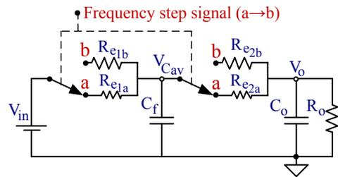
Figure 8. Average model of the 1:1 SCC for simulating a step change in switching frequency. State "a" is an initial state with equivalent resistance of  $R_{e,ia}$  ( $i = 1,2$ ), state "b" is after the frequency step with equivalent resistance of  $R_{e,ib}$ .
