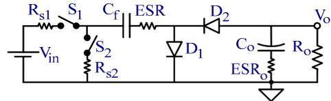
Figure 13. The demonstrated SCC (Inverting, 1:1 ratio).
