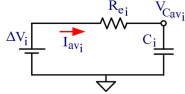
Figure 5. Generic average equivalent subcircuit.
