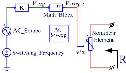
Figure 11. Implementation of dependent equivalent resistance in PSIM.
