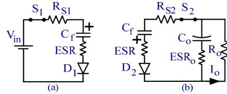
Figure 14. Inverting 1:1 SCC, instantaneous subcircuits: (a) Charging ( $i = 1$ ), (b) Discharging ( $i = 2$ ).
