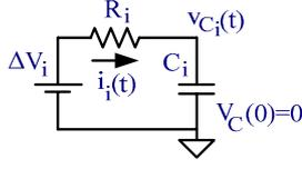
Figure 2. The generic capacitor-charging equivalent circuit.
