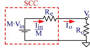
Figure 7. Static equivalent circuit of SCC.
