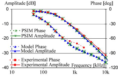
Figure 16. Input ( $v_{in}$ ) to output ( $v_o$ ) response (audio susceptibility) of the unity SCC of Fig. 1. Asterisks – Full circuit simulation results; Triangles – Traces of the Average model based analytical derivation (10); Squares - Experimental results; Solid traces – Amplitude response; Dashed traces – Phase response.
