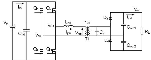
Figure 2. Parallel resonant converter with output voltage doubler.
