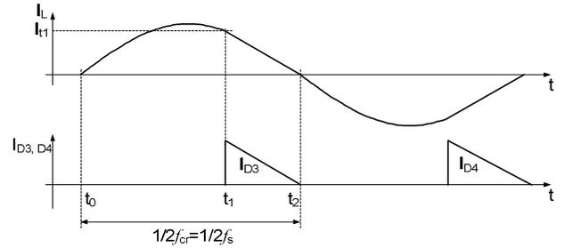
Figure 6. Inductor and output diode current of the converter with series diodes while operating at  $f_s = f_{cr}$ .
