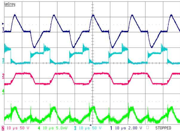
Figure 10. Typical experimental results. Loaded by magnetron.
