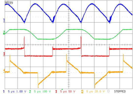
Figure 9. Experimental results. Resistive load ( $\sim 16 \text{ k}\Omega$ ). Upper trace: rectified inductor current  $100 \text{ A/div}$ . Second trace from the top: transformer's primary voltage  $100 \text{ V/div}$ . Third trace from the top: drain voltage of transistor Q3,  $50 \text{ V/div}$ . Lower trace:  $I_{D3}-I_{D4}$  (see Fig. 4)  $1 \text{ A/div}$ . Horizontal scale:  $5 \mu\text{s/div}$ .
