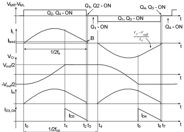
Figure 5. Key waveforms of the proposed converter.
