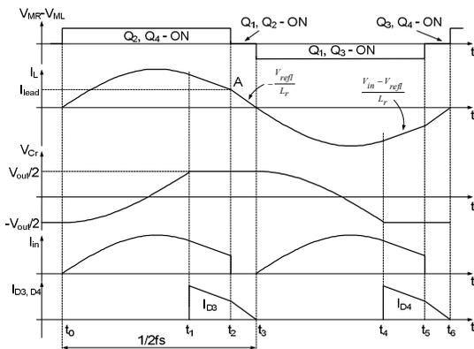
Figure 3. Key waveforms of the converter of Fig. 2
