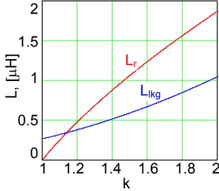
Figure 8. Leakage and resonance inductances for different  $k$ 's.
