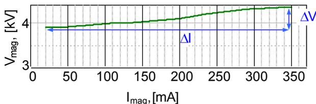
Figure 1. Output characteristic of magnetron.
