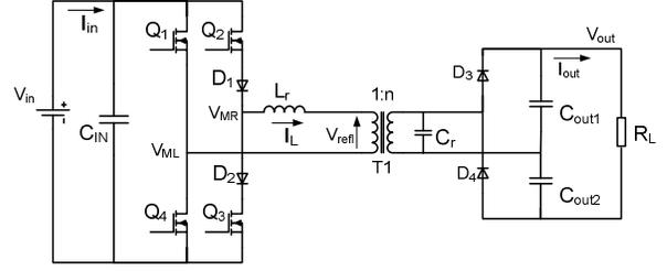
Figure 4. Proposed topology with input diodes.
